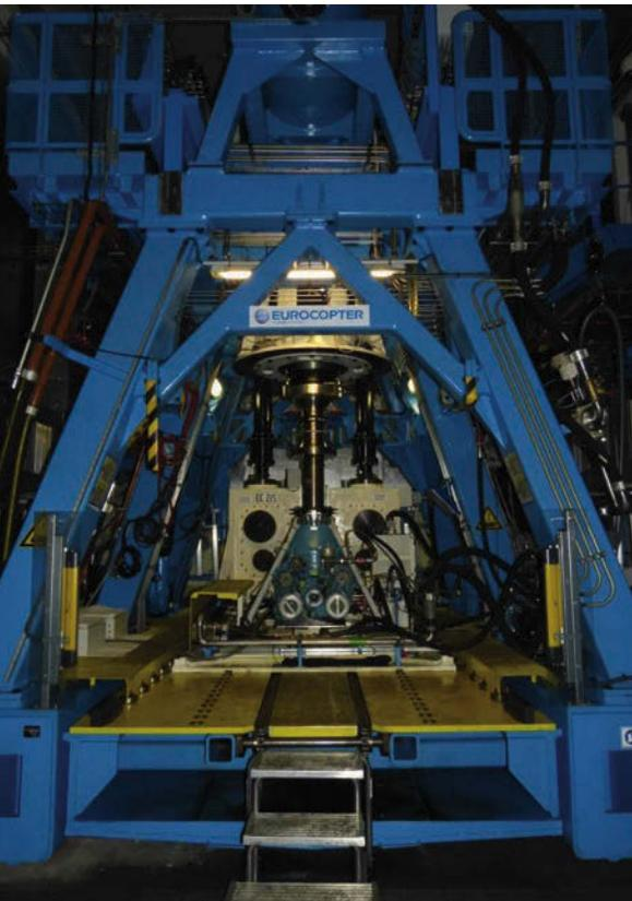
prototype and production components. In order to ensure that the dynamic flight loads acting on the shaft were consistent with the design parameters, the laboratory ran an EC225 MGB equipped with 32 strain gauges through a series of dynamic tests. After almost 400 hours of testing, the failure was reproduced.
