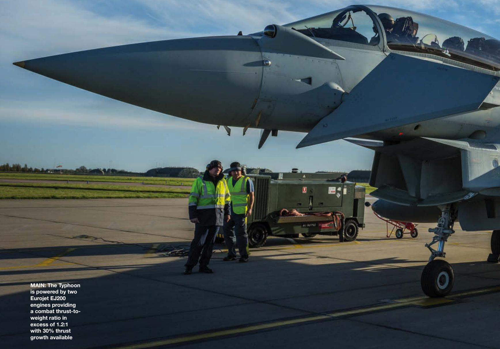
**MAIN:** The Typhoon is powered by two Eurojet EJ200 engines providing a combat thrust-to-weight ratio in excess of 1.2:1 with 30% thrust growth available
