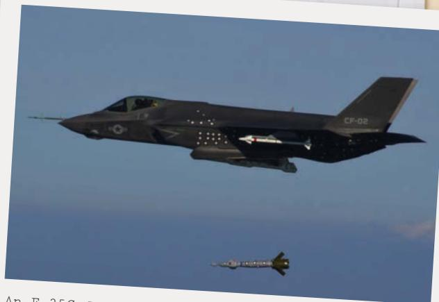
An F-35C Joint Strike Fighter from the Naval Air Warfare Center Aircraft Division at Patuxent River releases a 500 lb inert laser-guided bomb over the Atlantic Test Range. (Image: US Navy)
