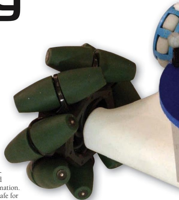
**MAIN:** A holonomic vehicle with Mecanum wheels has four independently controlled motors
