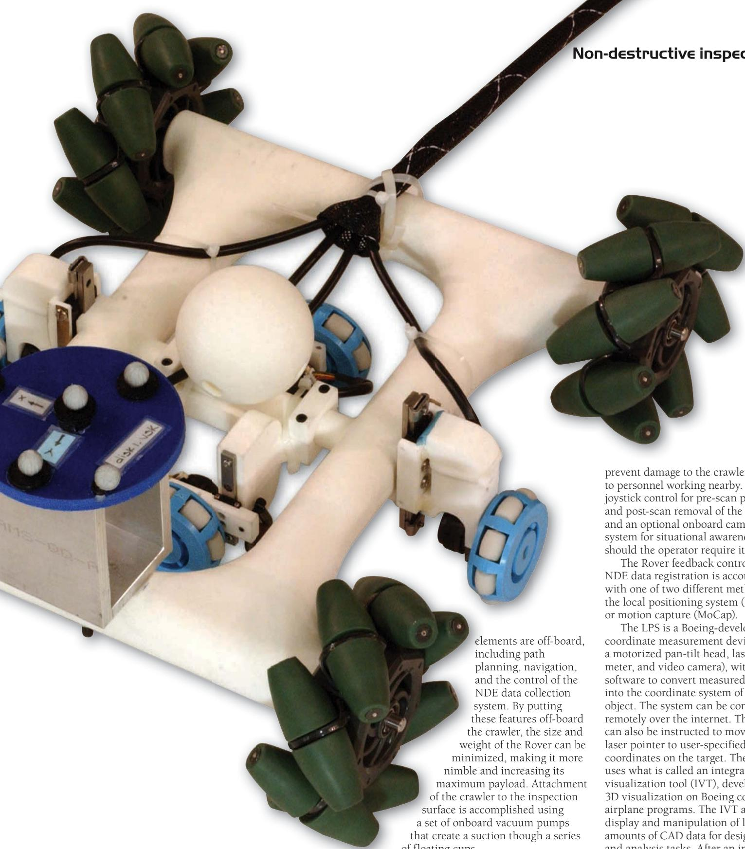
**“ATTACHMENT OF THE CRAWLER TO THE INSPECTION SURFACE IS ACCOMPLISHED USING A SET OF ONBOARD VACUUM PUMPS”**
