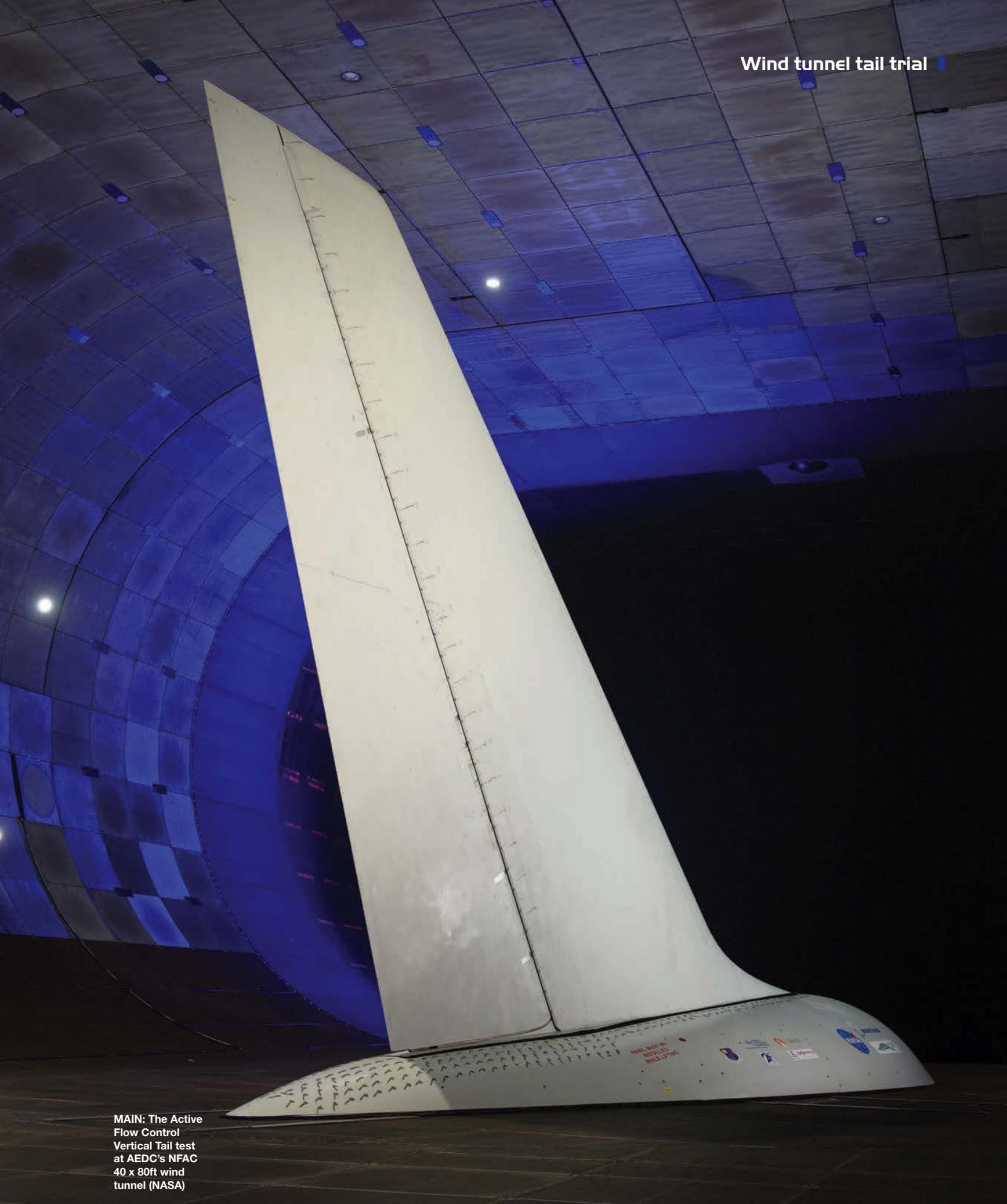
MAIN: The Active Flow Control Vertical Tail test at AEDC's NFAC 40 x 80ft wind tunnel (NASA)
