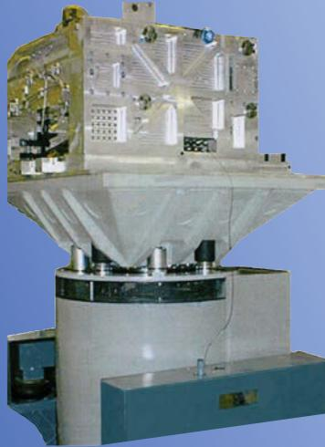
Unholtz-Dickie's revolutionary ***Induct-A-Ring (IAR)*** Shaker with its single turn solid metal driver coil armature has become the industry standard in its class.
