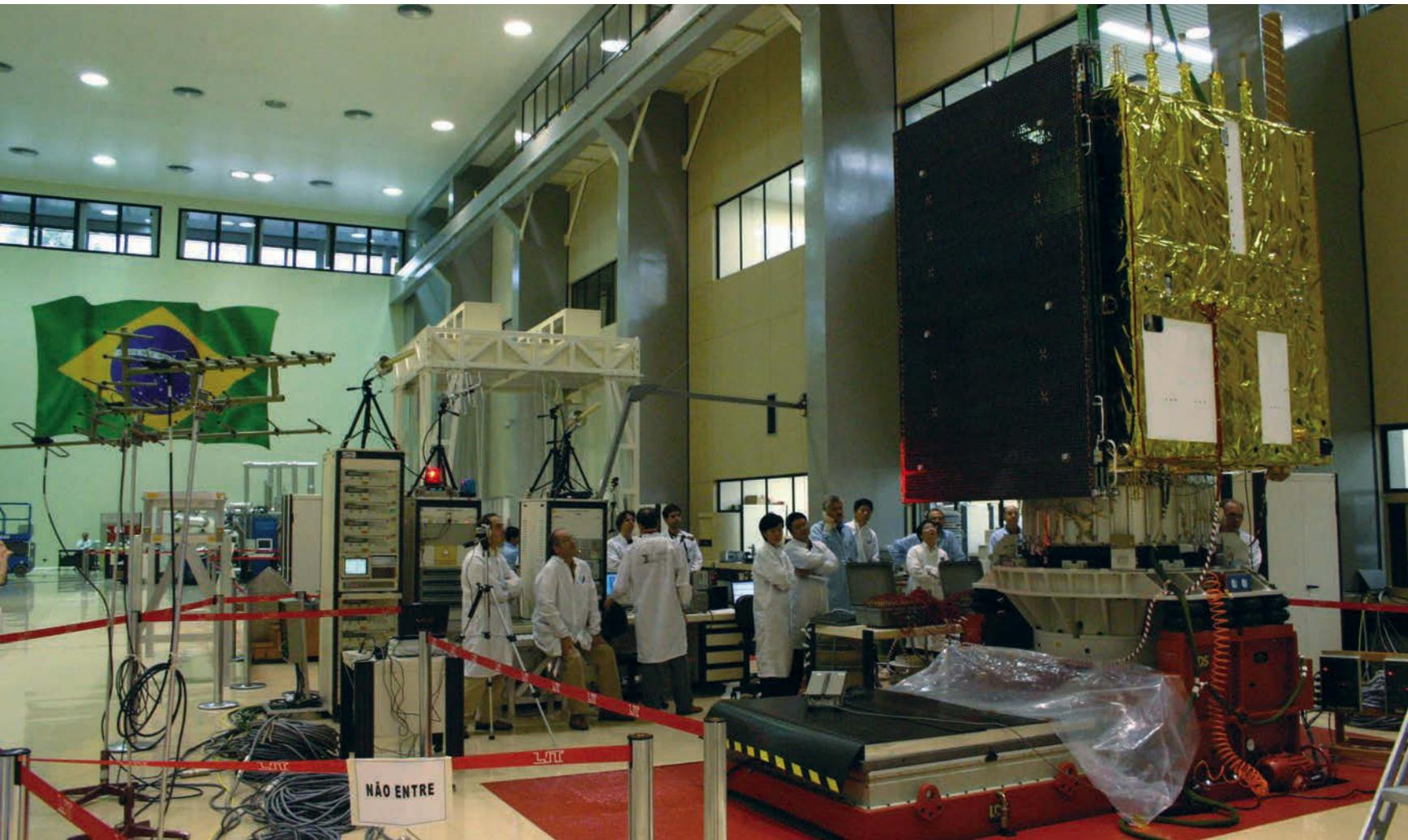
A satellite sits on an LDS shaker, using a custom adapter that reproduces the interaction between the satellite and its launcher, measuring the force interaction with embedded transducers
