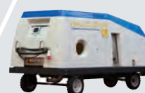
> Waste Line Cleaning Trolley
