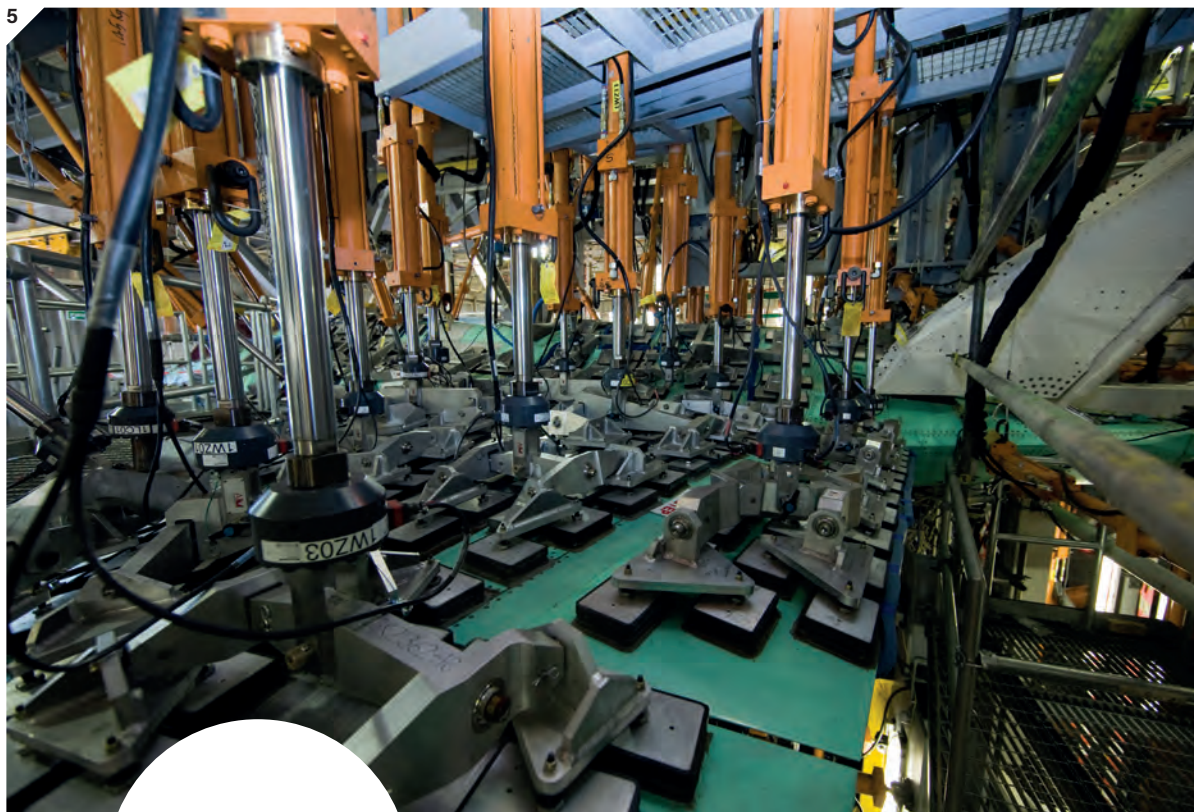
5 // The 350 ton test rig was built to 'fly' the F-35 Lightning II through a series of flight scenarios
