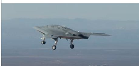
California and landed autonomously near a pre-determined touchdown point to simulate a tailhook-arrested landing on a carrier. The Office of the Secretary of Defense refocused the J-UCAS effort on Navy requirements in 2006, and Northrop Grumman won a contract in 2007 to design and build the 44,000 lb X-47B demonstrators.
