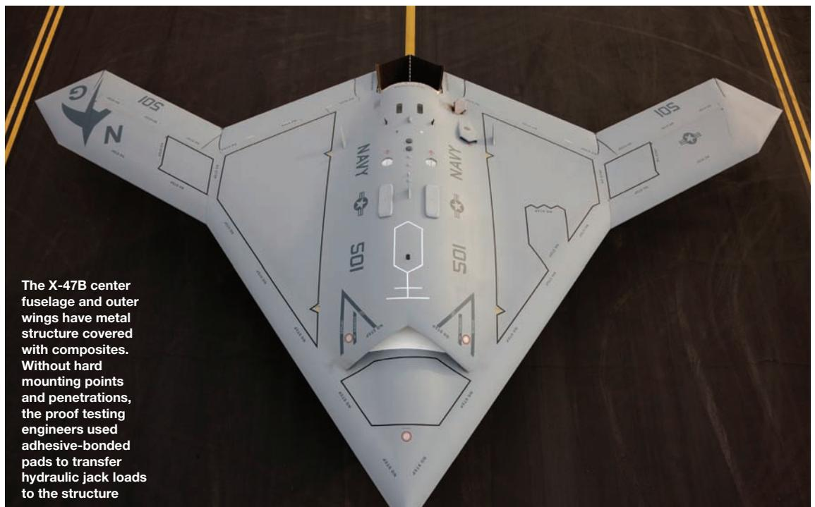
The X-47B center fuselage and outer wings have metal structure covered with composites. Without hard mounting points and penetrations, the proof testing engineers used adhesive-bonded pads to transfer hydraulic jack loads to the structure
