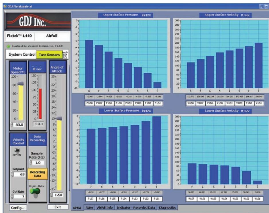
National Instruments LabVIEW Screen developed by Viewpoint Systems, Rochester, New York used to remotely control the wind tunnel while retrieving real-time data
