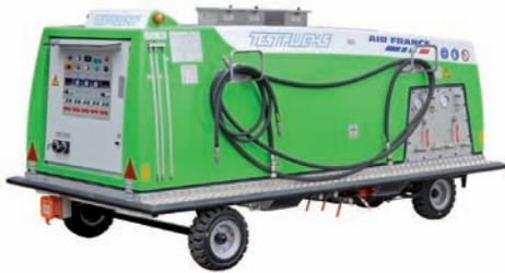
in the taxi phase, when engines may be contaminated by the aspiration of various substances like dust, sand, and hydrocarbons, causing higher fuel consumption and CO<sub>2</sub> output. This is why all major engine producers have established sophisticated washing procedures reducing a.m. effects and extending the lifecycle of engines.
