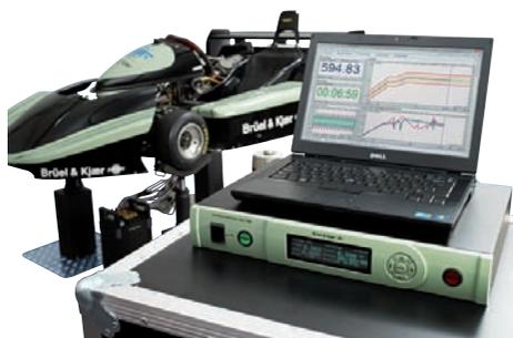
Having one complete system for vibration and data acquisition simplifies the test setup process as the same setup can be used for qualification and structural analysis, and simultaneously record data.
