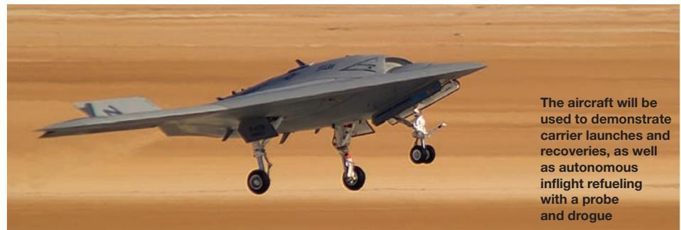
**The aircraft will be used to demonstrate carrier launches and recoveries, as well as autonomous inflight refueling with a probe and drogue**
