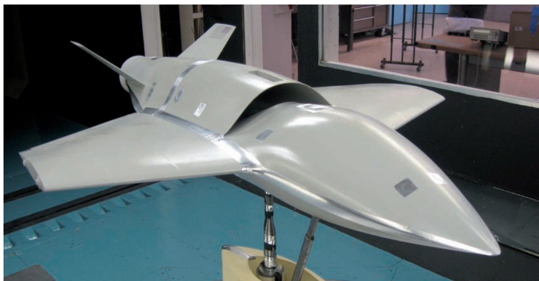
The AD-150 wind tunnel model with high control surface deflection, and during construction
