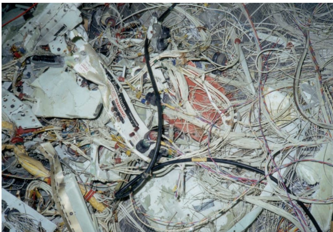
Above: The search for a crack in the wire from the huge piles recovered from TWA 800
