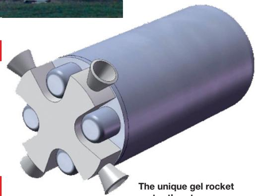
The unique gel rocket motor thrusters
