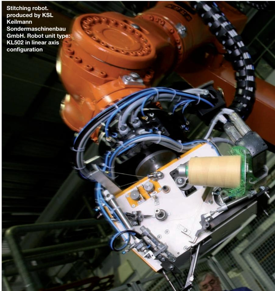
**Stitching robot, produced by KSL Keilmann Sondermaschinenbau GmbH. Robot unit type: KL502 in linear axis configuration**
