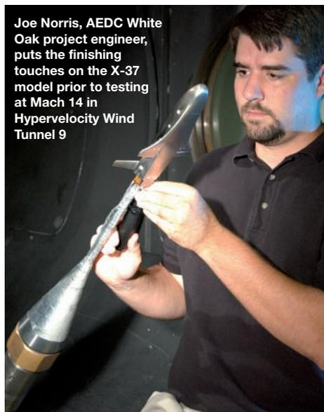
Joe Norris, AEDC White Oak project engineer, puts the finishing touches on the X-37 model prior to testing at Mach 14 in Hypervelocity Wind Tunnel 9
