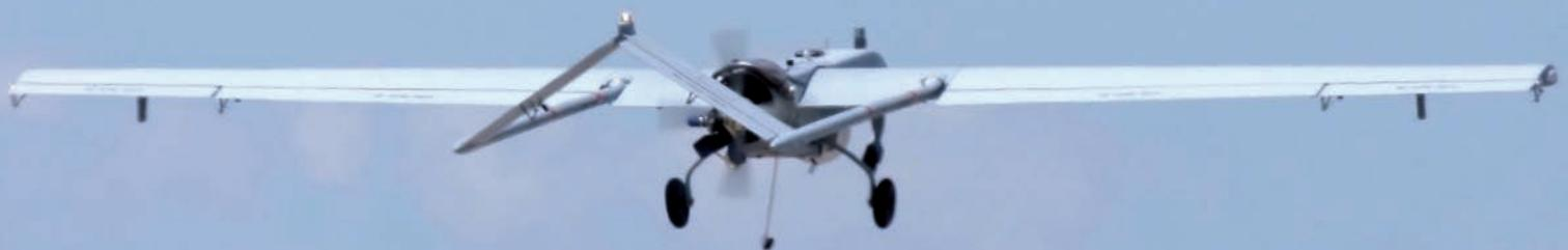
The aircraft can see targets up to 125km away from the tactical operations center, and recognize vehicles from 8,000ft
