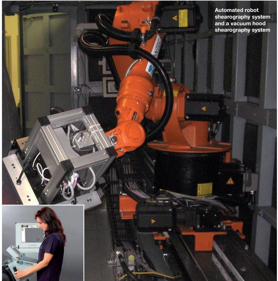
Automated robot shearography system and a vacuum hood shearography system
