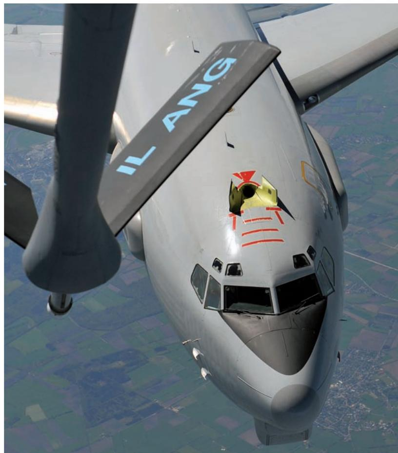
In May 2010 corrosion on the E-3A was detected. After repair work to the nose landing gear door and tests, the aircraft were back in the air within a week
