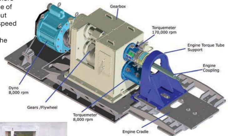
ABOVE: Dual output shaft gearbox with integral flywheel
