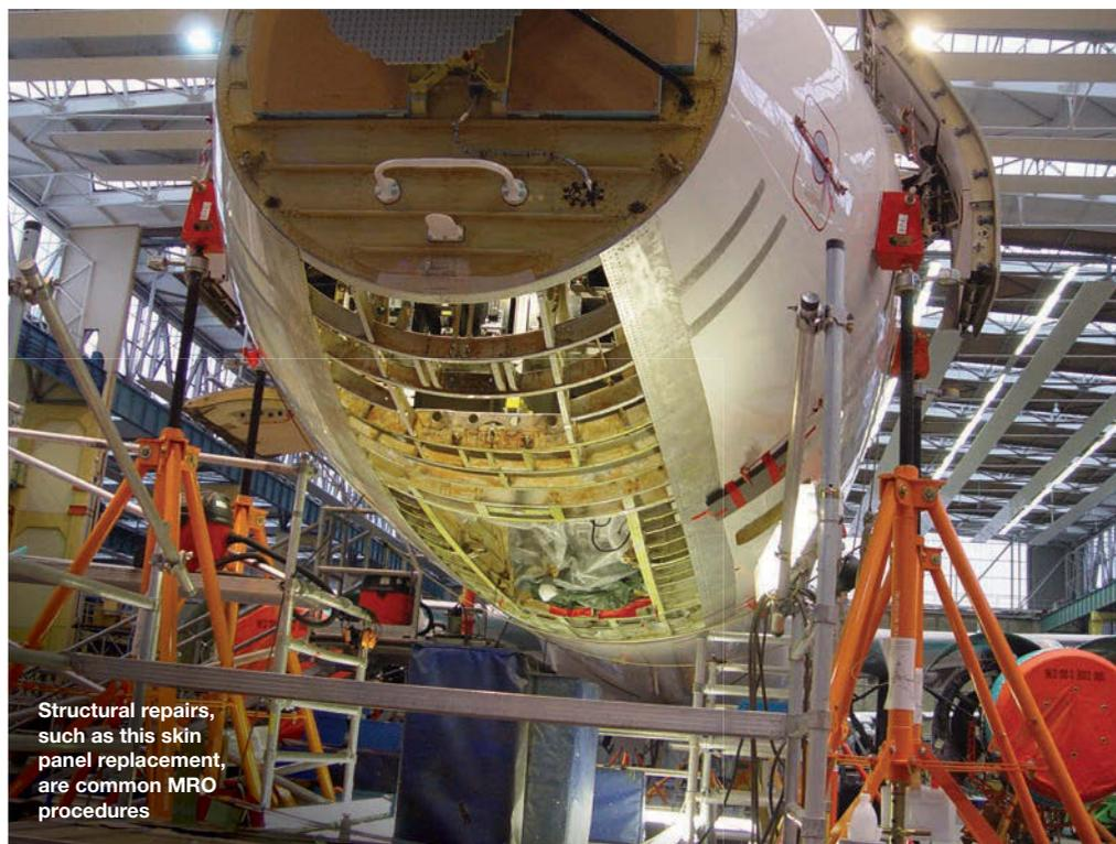
Structural repairs, such as this skin panel replacement, are common MRO procedures
