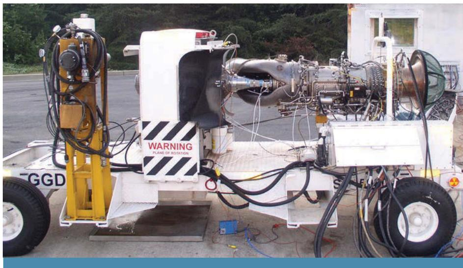
LEFT: Varoc air dyno testing a T58 engine
