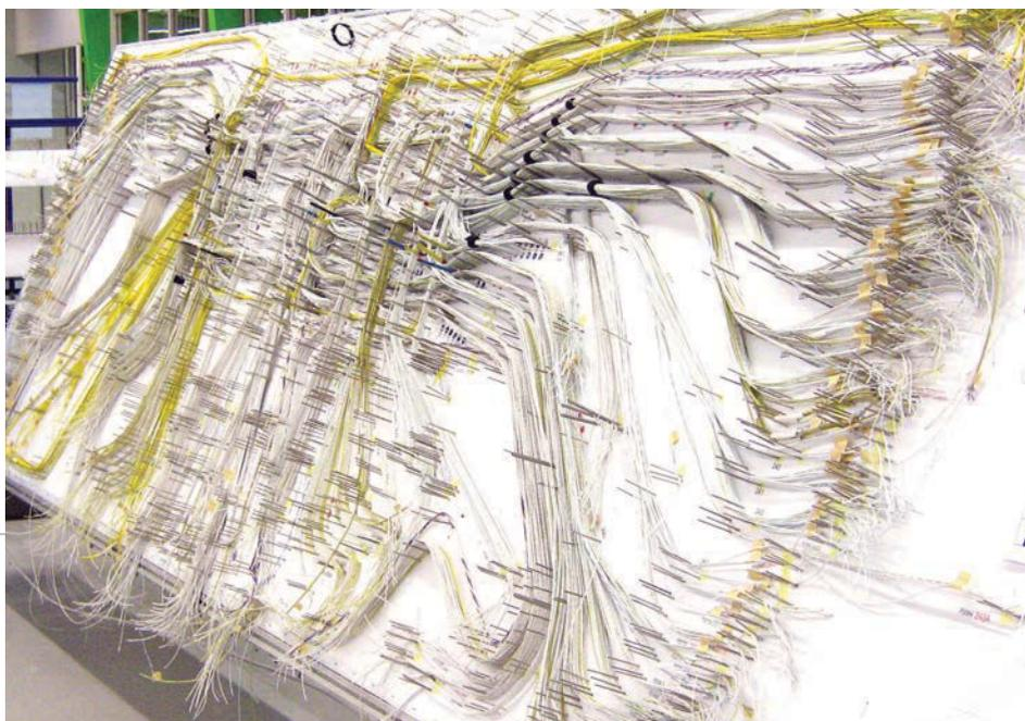
ABOVE LEFT/LEFT: Visual inspection of each termination verifies the correct components and markings. Fokker designs form boards used to assemble the wire harnesses
