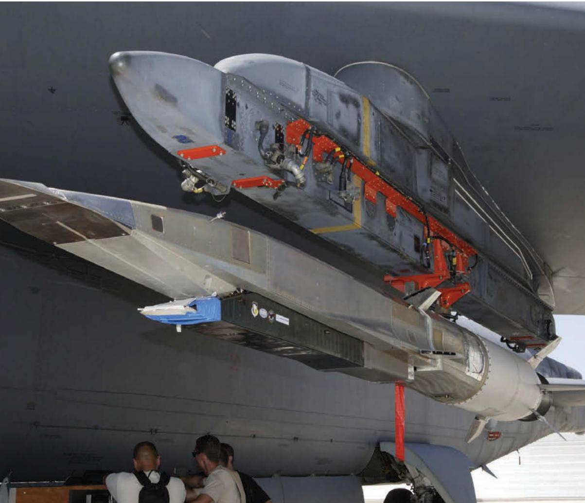
**ABOVE: The WaveRider, developed by Boeing, DARPA and the US Air Force, is designed to test the feasibility of Scramjet flight**
