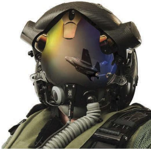
**ABOVE: The HMDS displays head-steerable symbology – the pilot’s line of sight dictates the content that appears on the visor**
