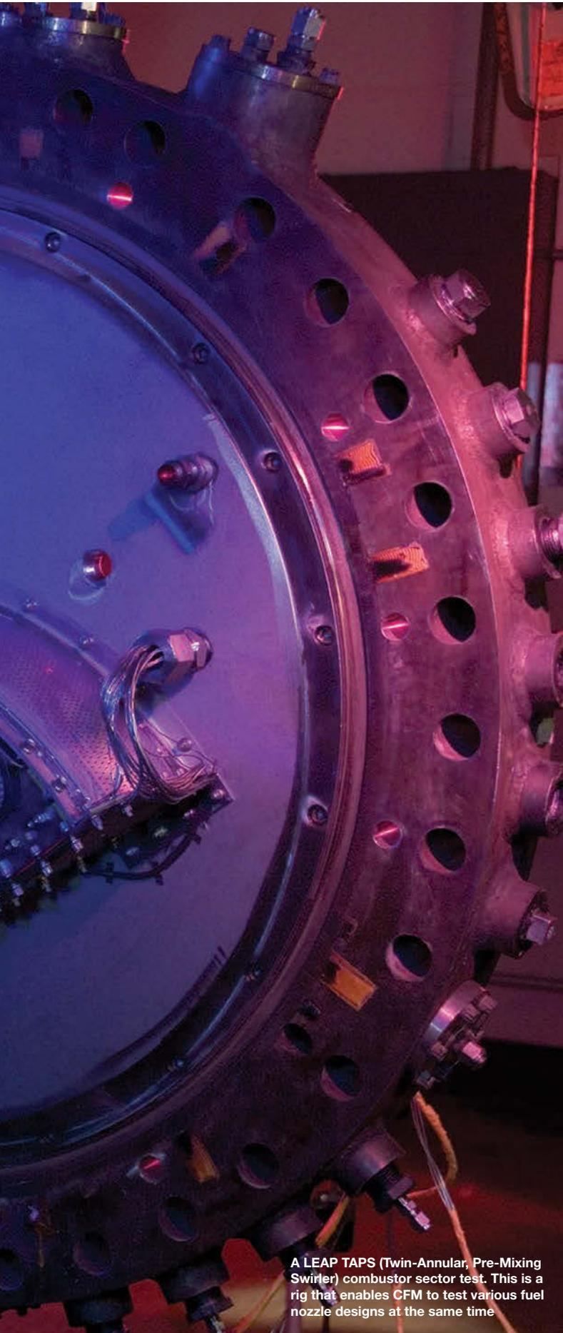
A LEAP TAPS (Twin-Annular, Pre-Mixing Swirler) combustor sector test. This is a rig that enables CFM to test various fuel nozzle designs at the same time
