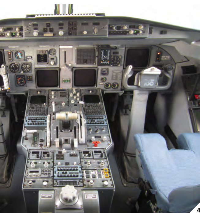
4 // Instrumented captain's control wheel and flight test display
