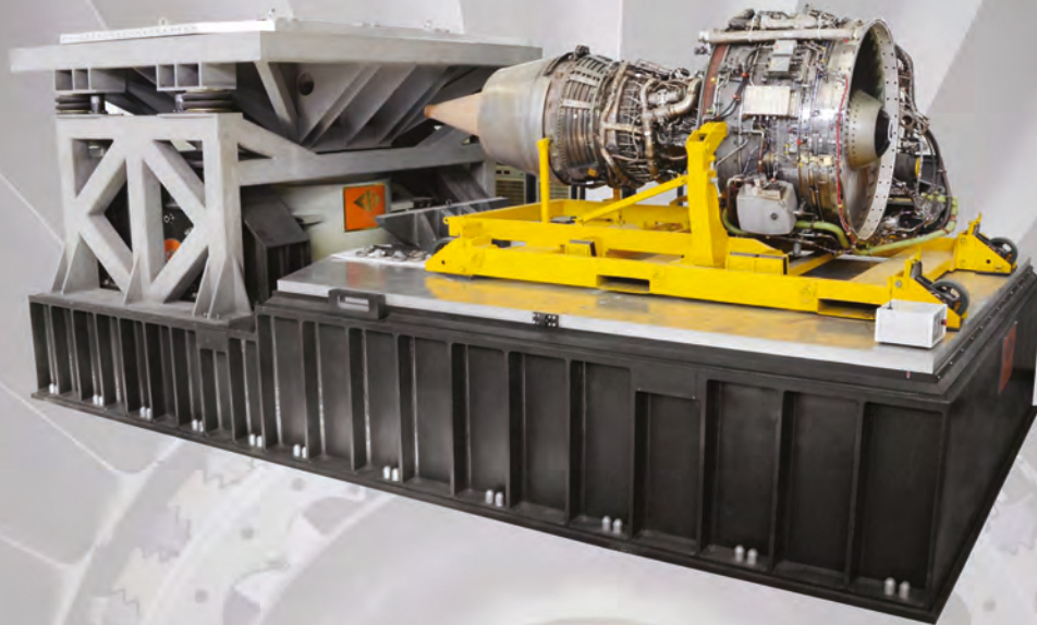
600 KN Force Rated Electrodynamic Shaker
