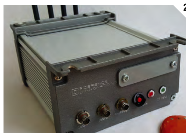
2 // The NIFTI sensors send information using bespoke wireless technology to a unit mounted in a pod, which is typically carried on an external hardpoint
