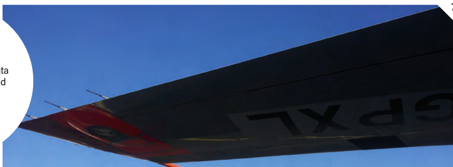
9 // The air data computer inside the ADB recorded angle of attack, slip, total and static pressure, and total air temperature
