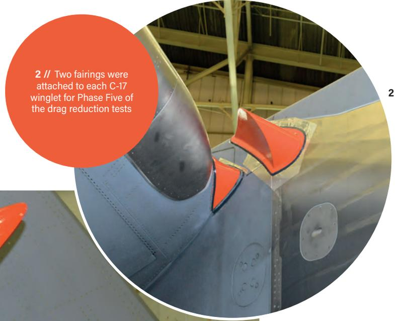
2 // Two fairings were attached to each C-17 winglet for Phase Five of the drag reduction tests
