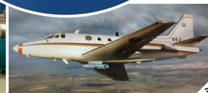
including centerline and wingtip positions. For installation of optical sensor heads and turrets, the aircraft also has a through-mounting hole in the belly centerline. The cabin can house several racks of flight test instrumentation as well as operator consoles for flight test engineers and technical subject matter experts.
