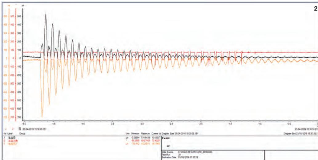
2 // Strain test data using m+p Coda showing the principle strain 1, principle strain 2 and the angle of principle direction
