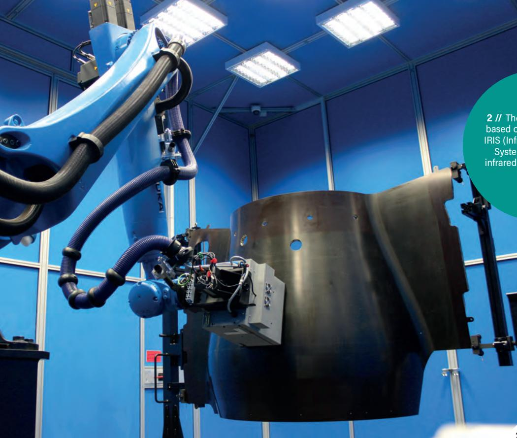
2 // The NDT process is based on a robot named IRIS (Infra Red Inspection System), which uses infrared thermography to read data
