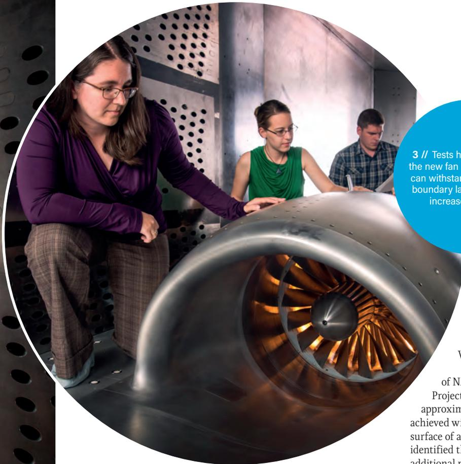
3 // Tests have shown that the new fan and inlet design can withstand the turbulent boundary layer airflow and increase efficiency
