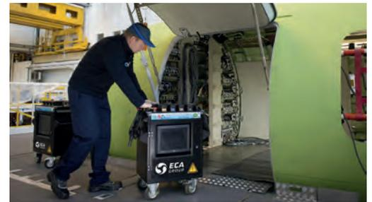
ECA Group has developed its novel 'T-Cell' technology to solve challenges with mixed hardware in test benches, component obsolescence and software issues due to operating system upgrades.
