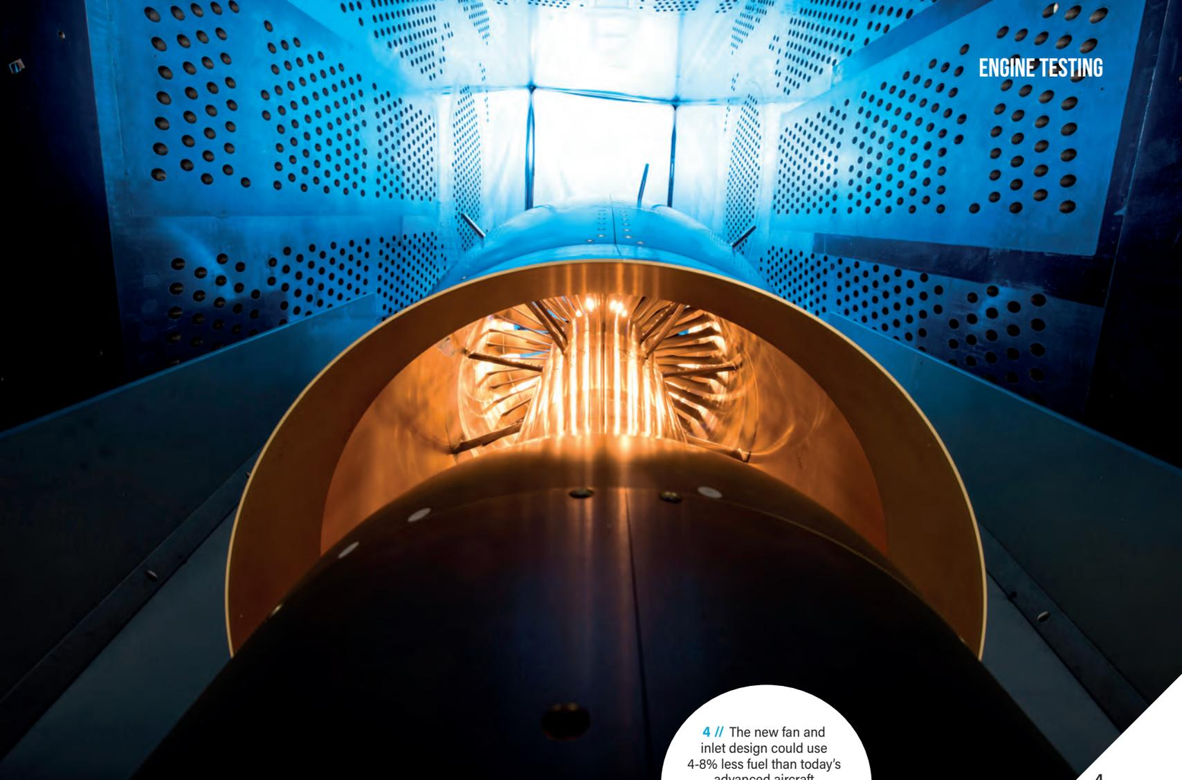
**4 //** The new fan and inlet design could use 4-8% less fuel than today's advanced aircraft
