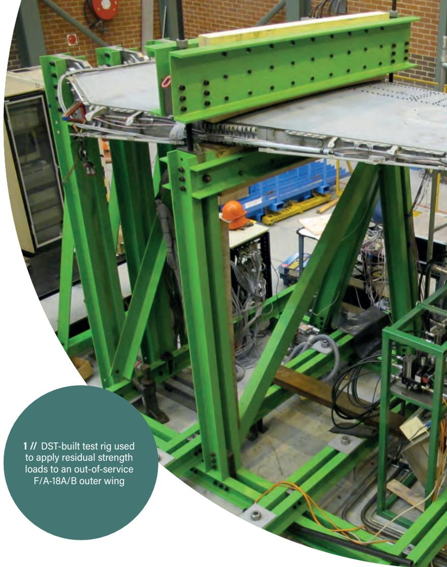
1 // DST-built test rig used to apply residual strength loads to an out-of-service F/A-18A/B outer wing
