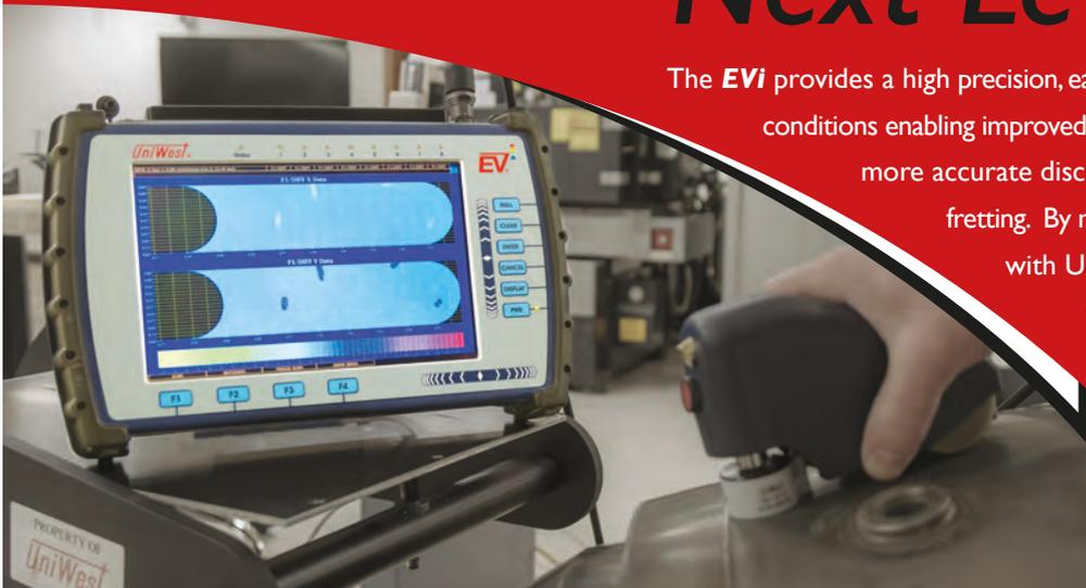
The **EVI** provides a high precision, easily readable display of surface conditions enabling improved interpretation of data while giving more accurate discernment of cracks, pits, gouges and fretting. By merging innovative surface imaging with UniWest's renowned, best-in-class signal to noise the **EVI** system sets a the standard of precision for eddy current testing in a portable and easy to use package.
