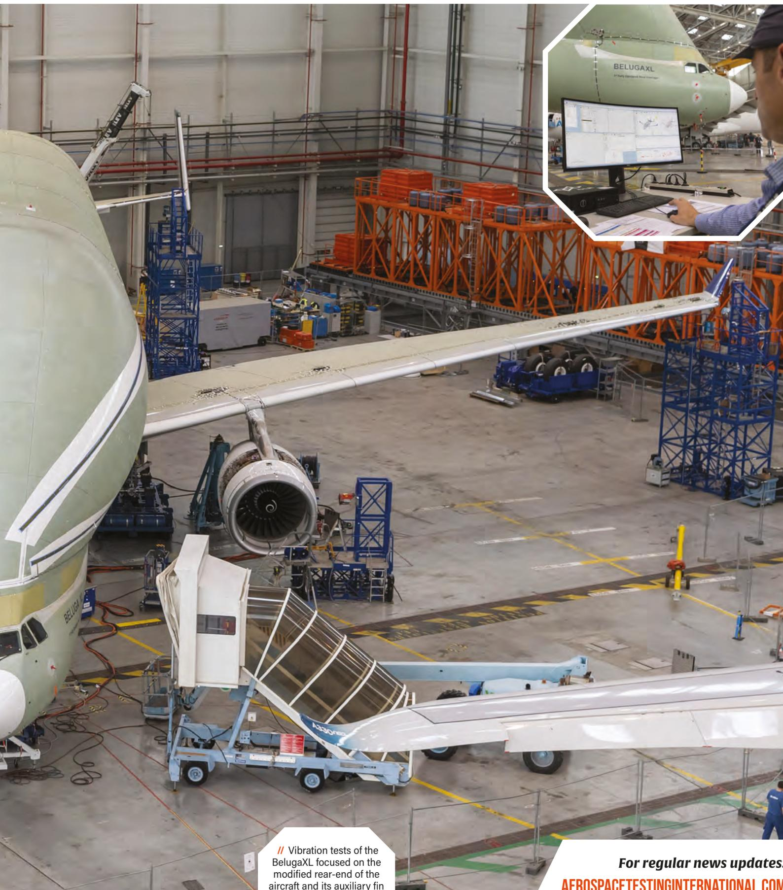
// Vibration tests of the BelugaXL focused on the modified rear-end of the aircraft and its auxiliary fin
