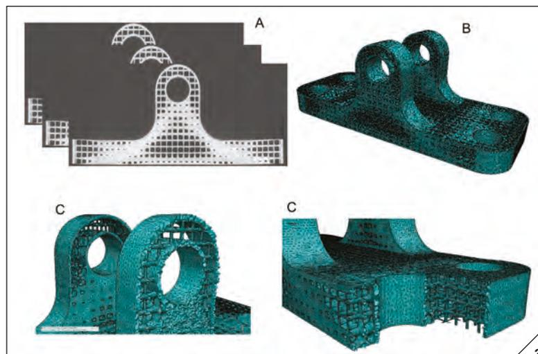
3 // (A) Representative stack of image data generated from CT scan of the bracket. (B) STL surface reconstruction. (C) Cross-sections of FE mesh
