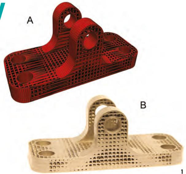
1 // (A) Final bracket design. (B) The AM titanium alloy bracket built using the laser powder bed AM machine
