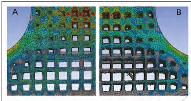
2 // Solved FE mesh on both the original design CAD (A) and the image-based FE mesh generated in Simpleware software (B)
