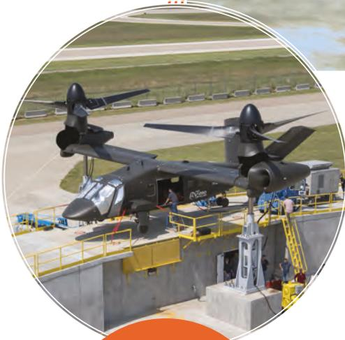
7 // The tiltrotor test stand built at the Bell Amarillo facility is designed to exercise the Valor through its complete tilt cycle from helicopter to airplane mode (Photo: Bell Helicopter)
