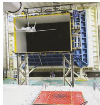
A recent two-week test campaign at the LLF in Marknesse has helped to develop a new tail for aircraft to reduce the engine noise of business jets. The U-tail works by shielding the engine from the ground and reflecting the noise upward.
