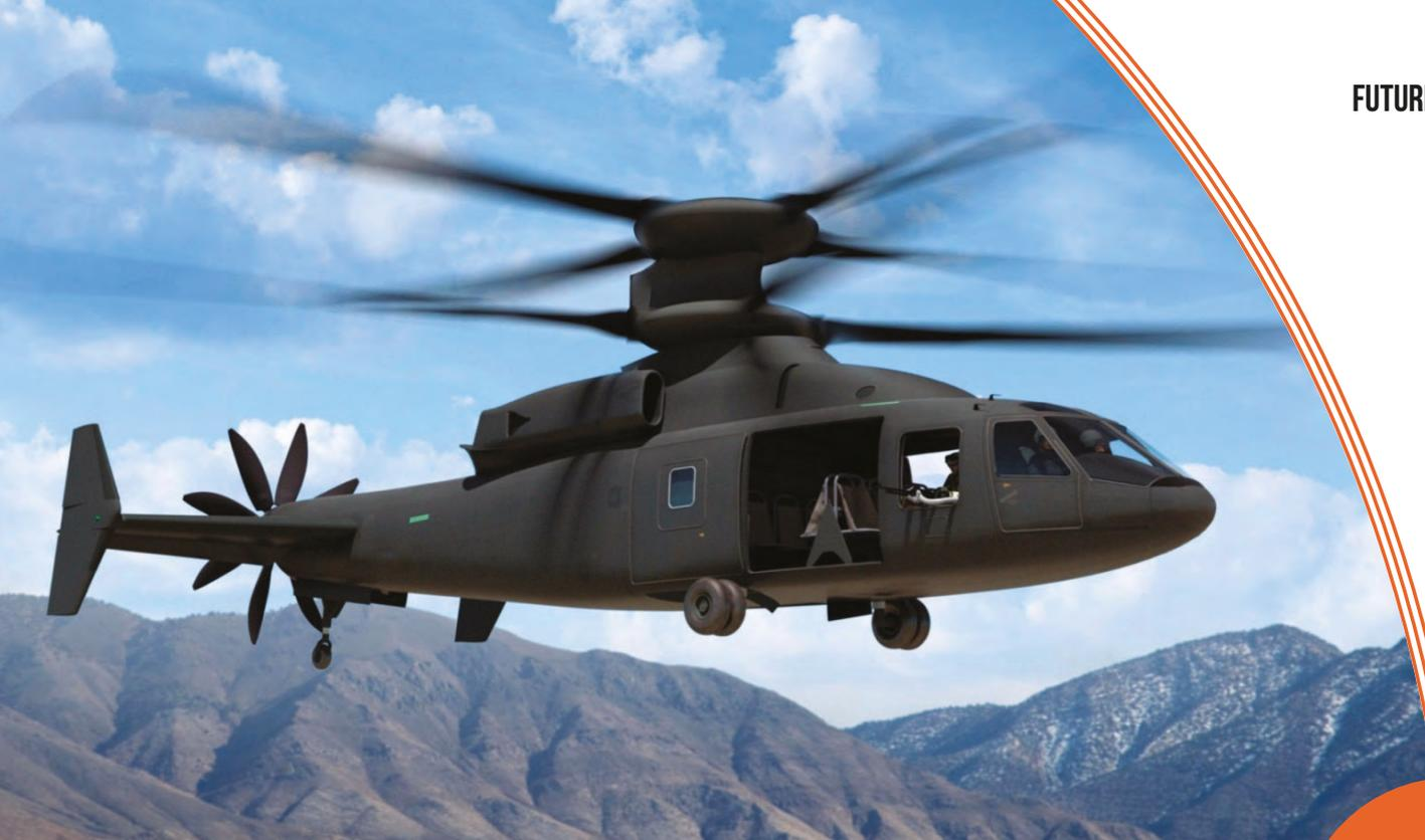
3 // The Sikorsky-Boeing SB-1 Defiant compound helicopter is sized to replace the UH-60 Black Hawk assault aircraft (Photo: Sikorsky)
