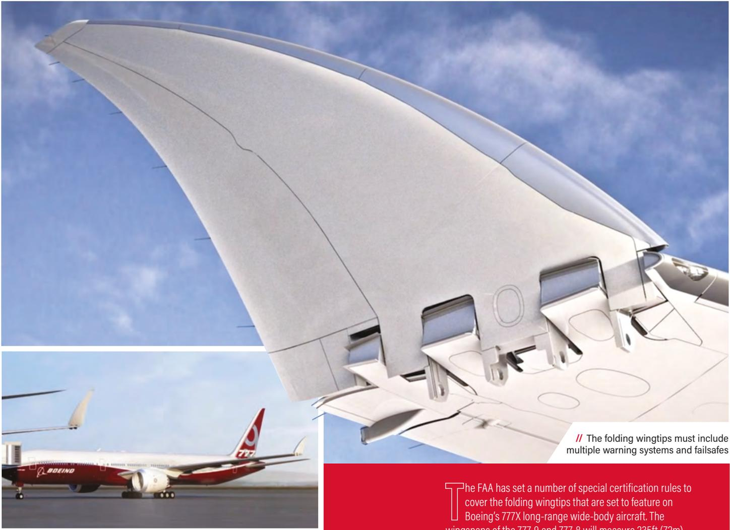
// The folding wingtips must include multiple warning systems and failsafes
