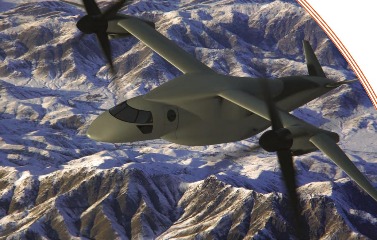
4 // Karem Aircraft expects ground runs of a full-scale Capability Set 3 Optimum Speed Tilt Rotor nacelle representative of its Maverick assault FVL in 2019 (Photo: Karem Aircraft)
