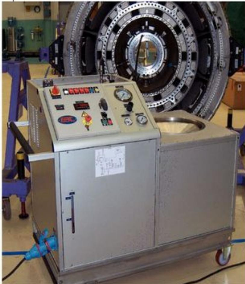
**Shock absorber test rig with the internal element of a two-systems hydraulic cart (below)**
