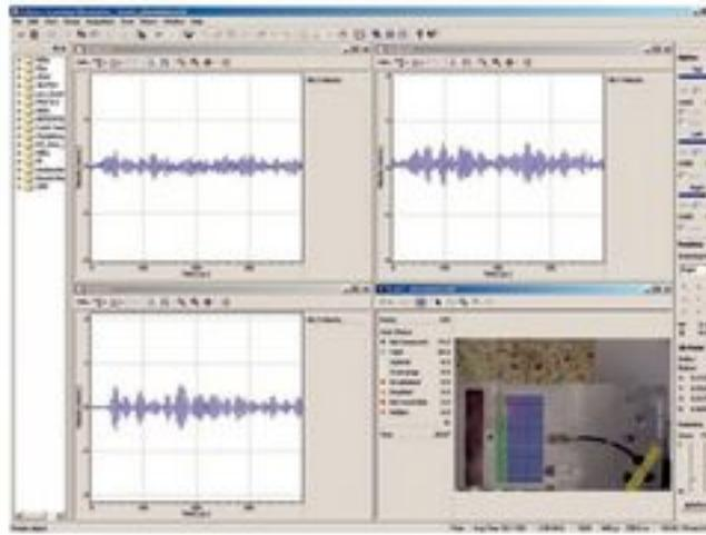
Experimental arrangements for lamb wave damage detection using 3D laser vibrometry as a receiver
