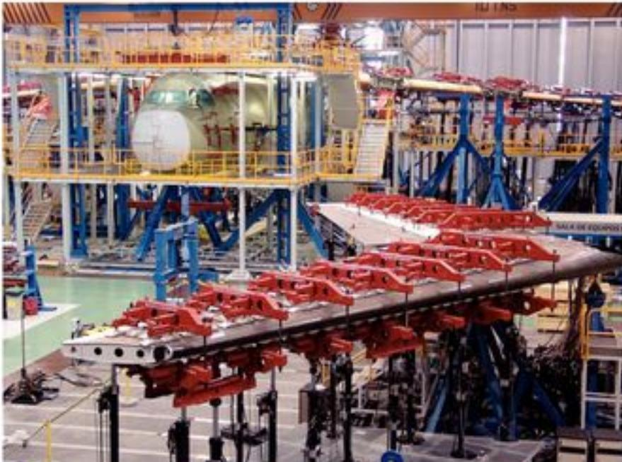
validates stress calculation methods by comparing measurements obtained from the test specimen with predictions from mathematical models. Engineers can then verify the performance of the airframe under simulated operational conditions by putting design theory into practice.
