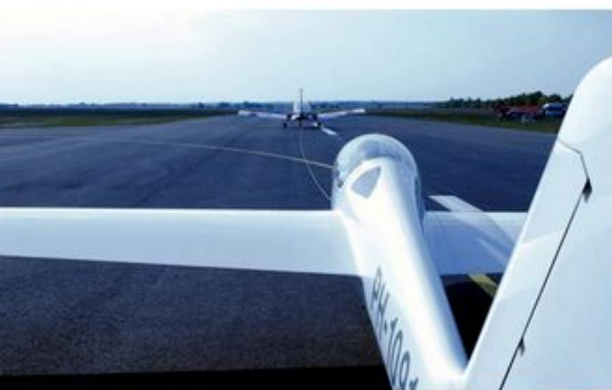
14m, which is quite short for a two-seater, but is needed for maneuverability. The maximum speed is 285km/h, and the allowed forces are from -6g to +9g. It is great to fly because the Fox does exactly what the pilot orders, but it is not easy to fly and one has to respect its limits. If the wing stalls, all the lift disappears immediately. Glider wings usually have a twist to maintain stability with decreasing speed for as long as possible, but on the Fox there is no twist.
