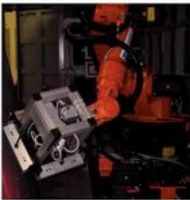
heat if necessary. Objects are illuminated with eight laser diodes and the shearography sensor reads out real-time phase stepping results. The system's interface is constructed for being easy to operate and harmonize with a company's written practice standard, in accordance with SNT-TC-1A or corresponding. The robot system can also be equipped with a software integrated sound excitation mode for vibration shearography through a piezo shaker or loudspeaker.
