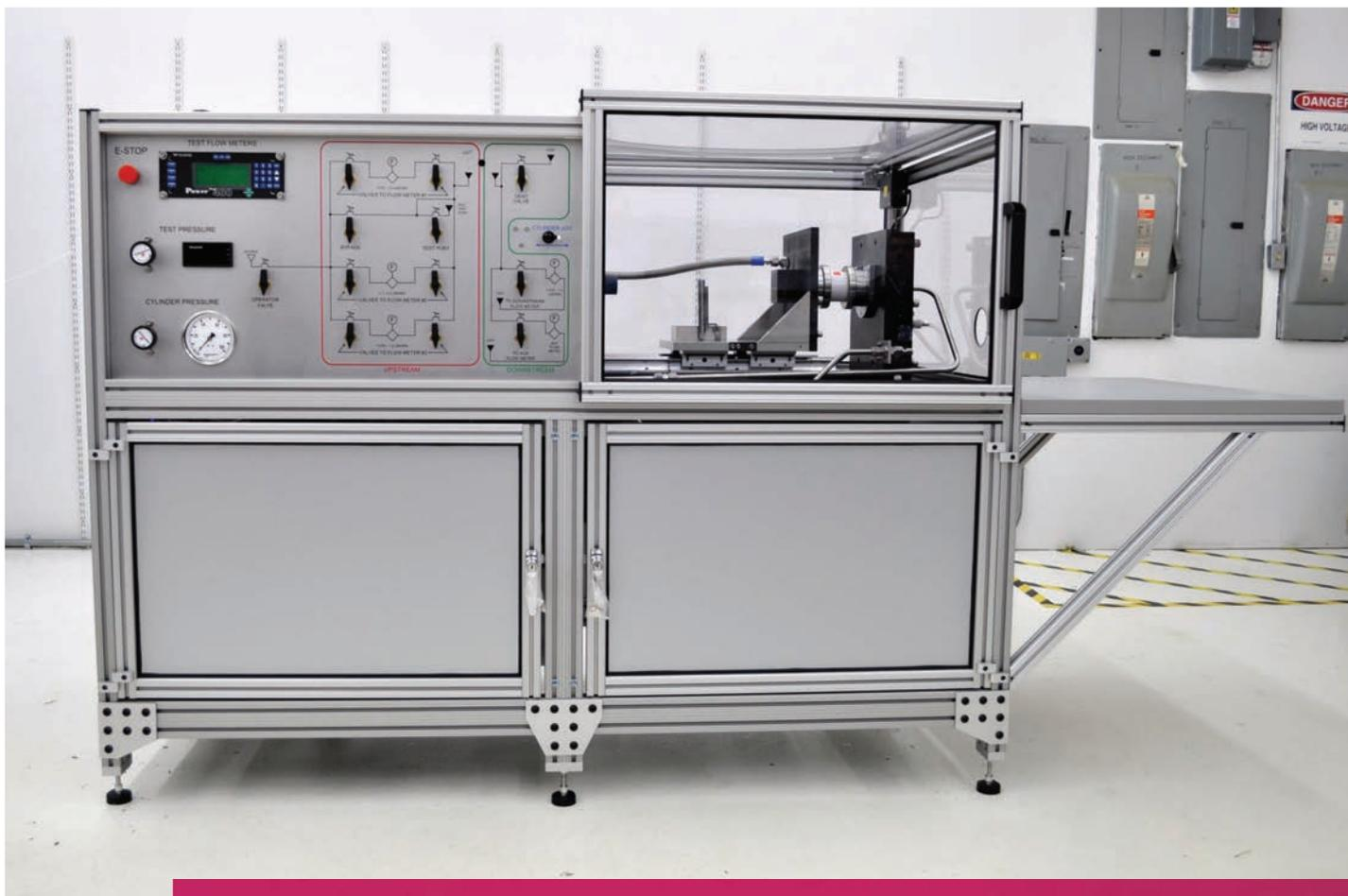
RIGHT: Valve tester at Kaney Aerospace, which also offers a thermal chamber with an ambient air temperature range of -75°C to 100°C, originally used to develop the 787's power electronics cooling system
