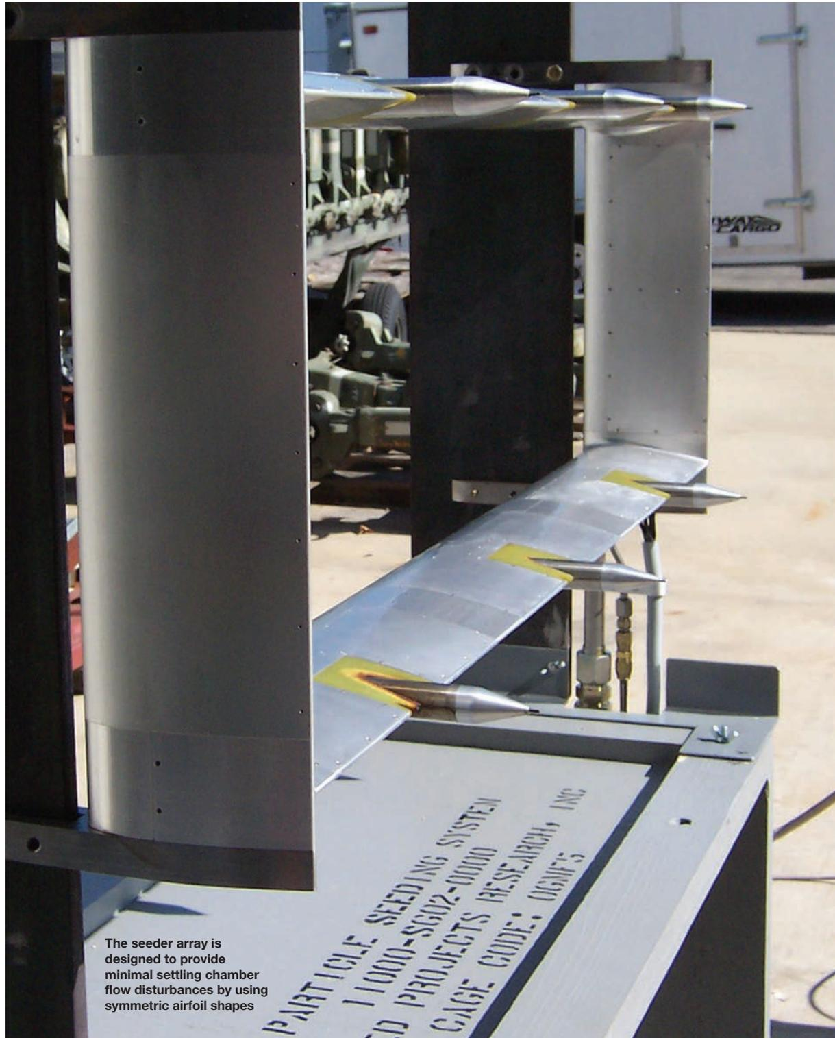
The seeder array is designed to provide minimal settling chamber flow disturbances by using symmetric airfoil shapes
