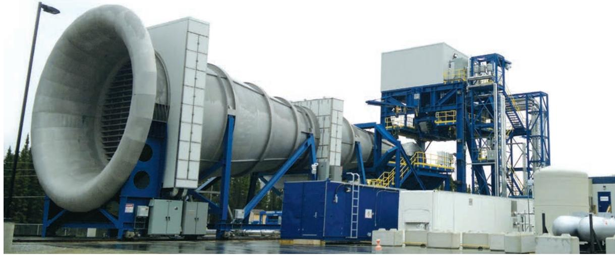
**ABOVE:** The 9m-diameter wind tunnel at the GLACIER facility in Canada can test engines with up to 150,000 lb thrust
