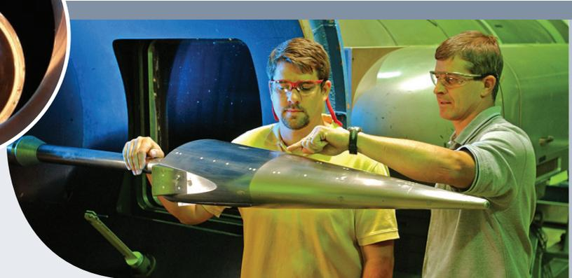
heating profiles and interrogation of boundary-layer transition using high-frequency microphones and pressure sensors. Taken together, this data product is being used to explain anomalies in flight and to reduce risk for upcoming flights.
