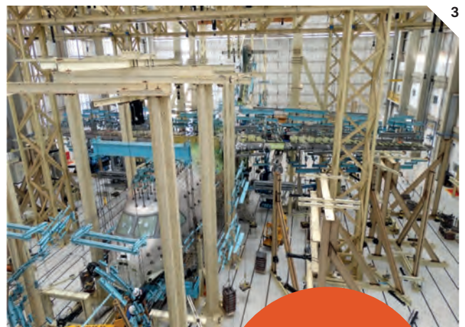
3 // Known within the company as Aircraft 801, this is the KC-390 structural test airframe
