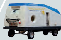
> Waste Line Cleaning Trolley
