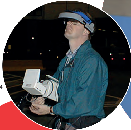
4 // Jeff Thompson early in his career, performing a field test to identify moisture ingress in 767 flap wedges using an infrared camera with a head-up display
