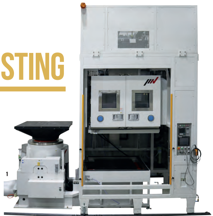
1 // Climatic chamber combined with a 65kN air-cooled shaker
