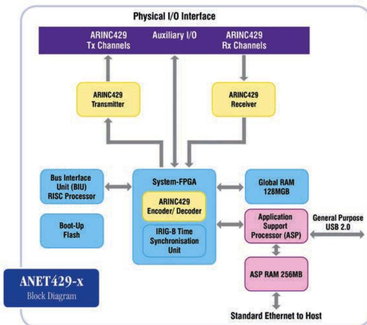
ABOVE: Block diagram of the Ethernet-based ARINC429 interface
