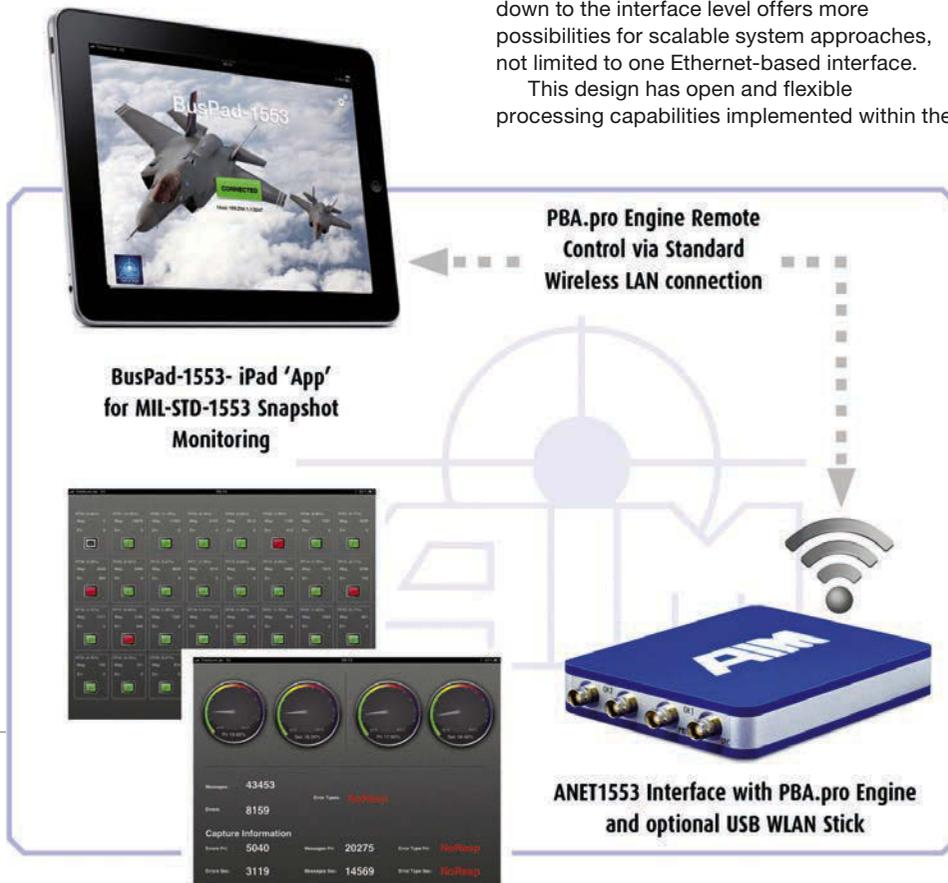
LEFT: Using an Ethernet-based interface wireless from a tablet
