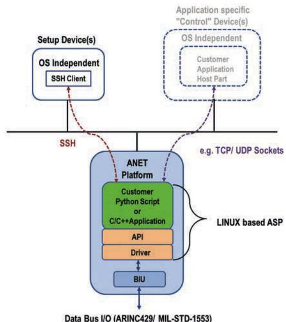
ABOVE: Software architecture of the Ethernet-based interface
