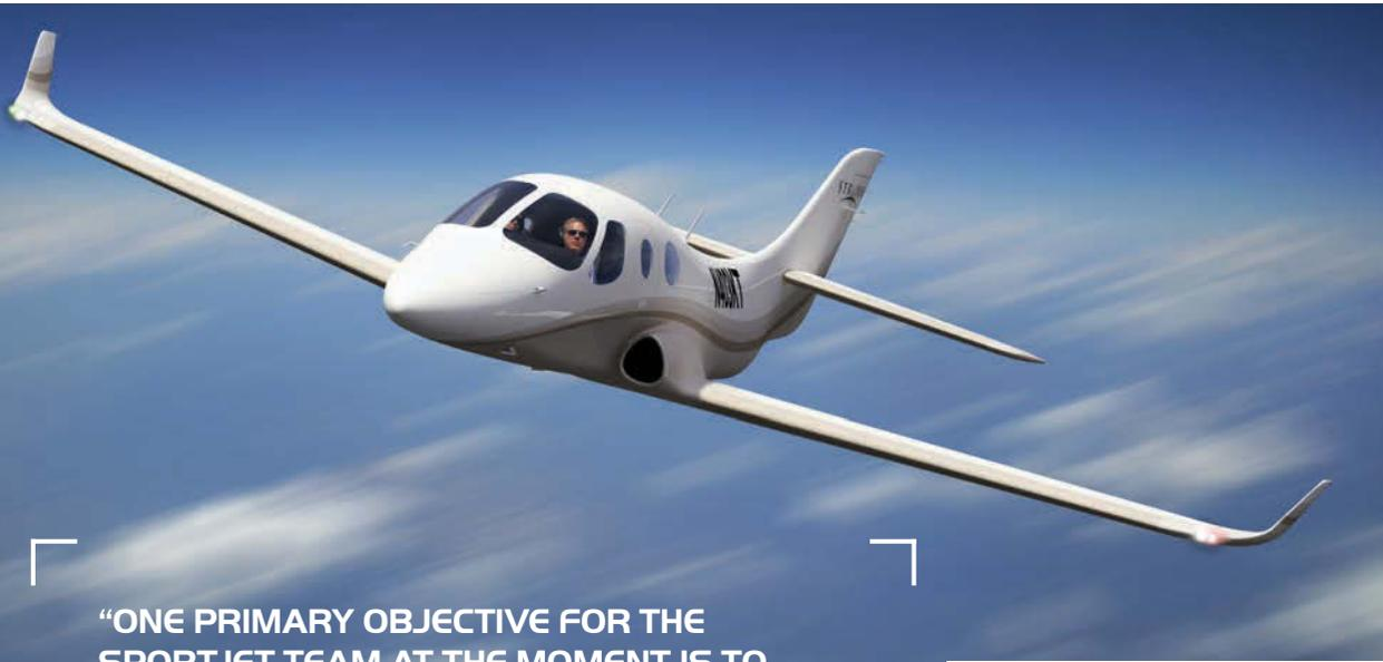
**LEFT:** The Stratos 714 has a length of just 38ft, take-off on a runway of only 600m, but can still fly at 415kts
