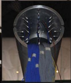
Series 112A shown installed in wind tunnel buffet model.
