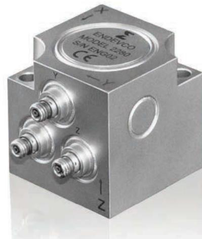
ABOVE: The 2280 is a hermetically sealed, triaxial, piezoelectric, charge-output accelerometer designed for high-temperature operations
