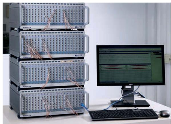
LMS vibration control systems can be expanded to hundreds of control, measurement and limiting channels. Users find it easy to use for routine random, shock, sine, and combined modes testing and have everything they need for state-of-the-art control and extensive data analysis.
