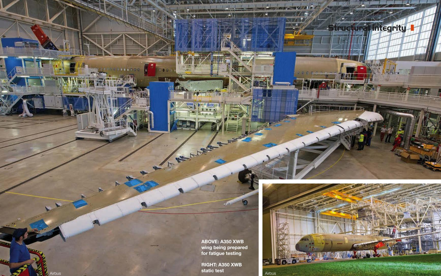
ABOVE: A350 XWB wing being prepared for fatigue testing
