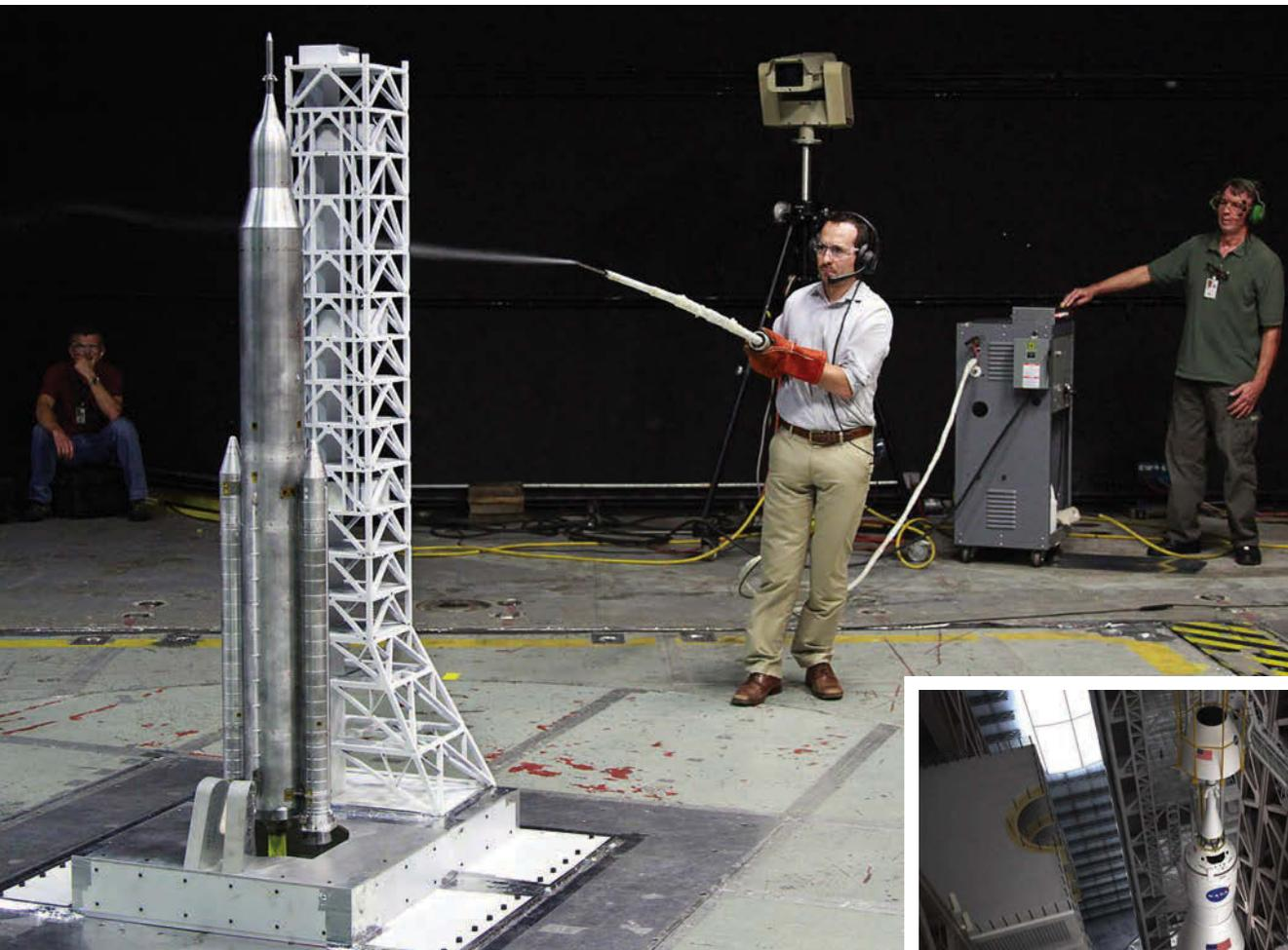
**LEFT: Engineers simulate changing ground wind conditions on a large-scale model of the SLS**
