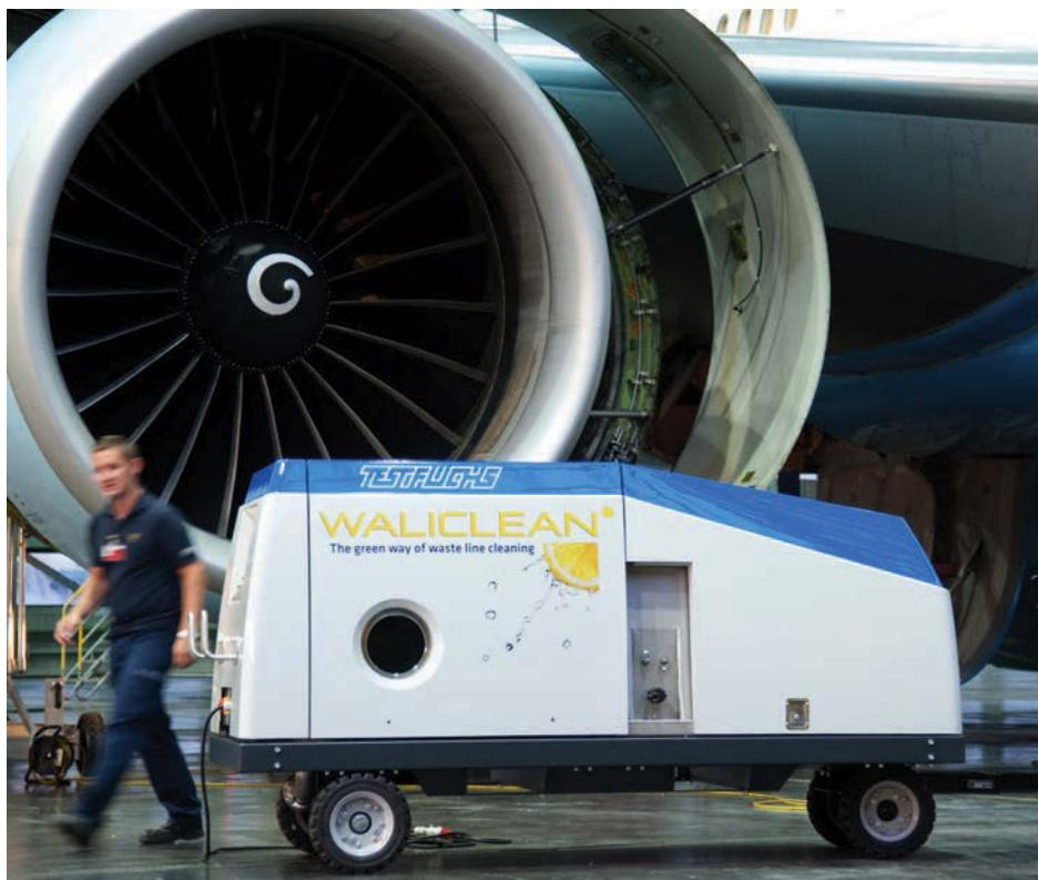
process starts, automatically stopping when finished. For safety reasons the Waliclean also performs a leakage check of the waste-line system. There is no need to monitor the cleaning process, which takes only five hours and can easily be performed overnight.
