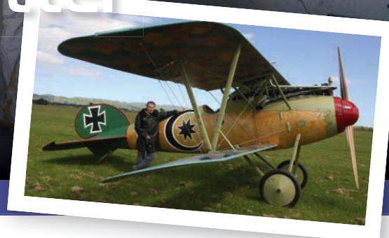
One of the most prolific aircraft manufacturers during World War I was Albatros, which created a series of single-seat fighters that were in service longer than all the Fokker fighters combined. The Albatros D.III introduced the distinctive 'V' strut-braced sesquiplane arrangement borrowed from the French Nieuport scouts.
