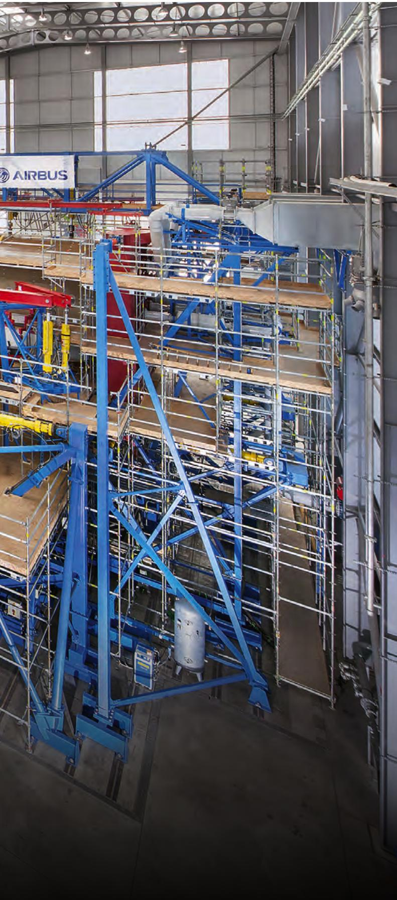
**LEFT: IABG simulated 86,400 A350 flights in the EF2 fatigue test rig at Erding**
