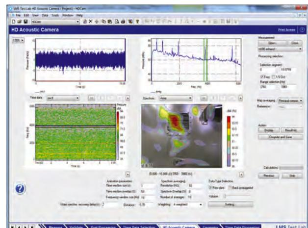
Pinpoint sound sources in seconds by combining the LMS Test.Lab™ High Definition Acoustic Camera, the LMS Circular Irregular Array with 45 microphones, and a compact 48-channel LMS SCADAS™ Recorder.
