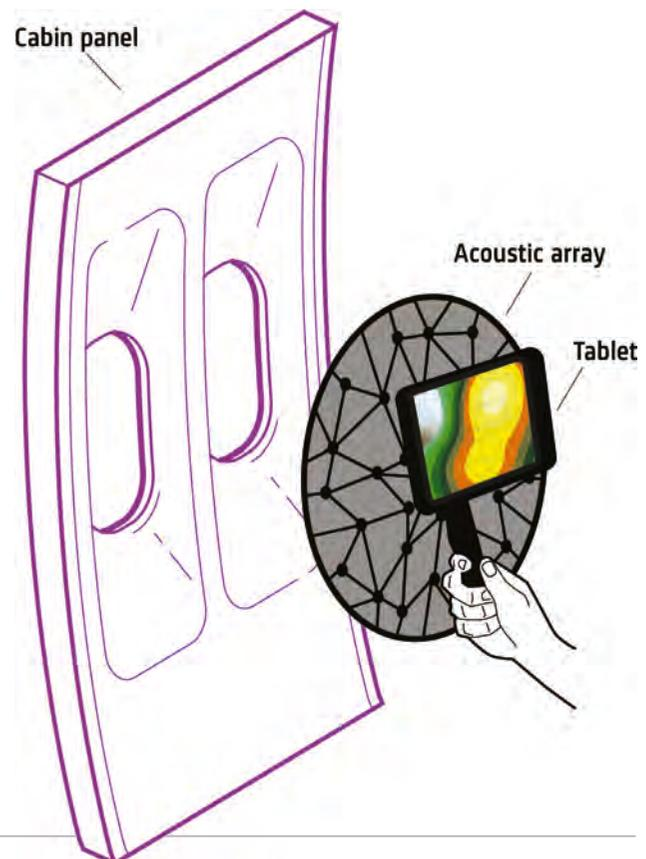
Brüel & Kjær's acoustic camera is a complete kit for mapping sound emissions in seconds
