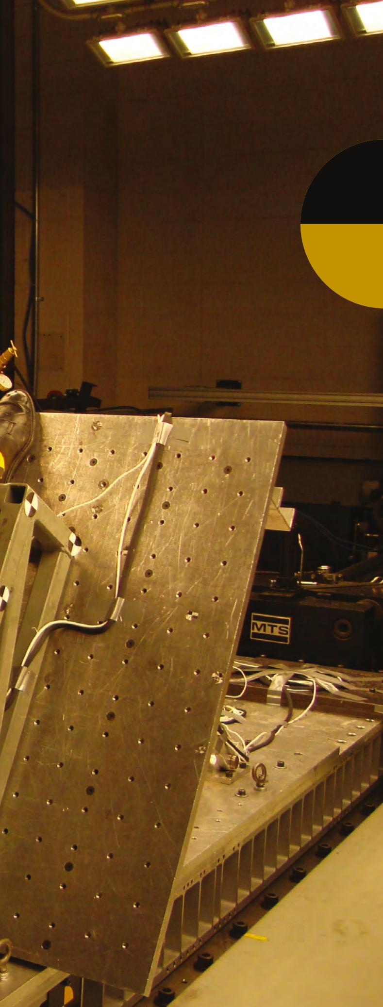
Aircraft seats are designed to remain intact during a deceleration of 16g – not far short of the impact of a top golfer's driver on the ball – without deforming to the extent that occupants would be seriously injured. And manufacturers are required not just to design them that way, but to demonstrate that seats, restraints and associated systems actually work.
