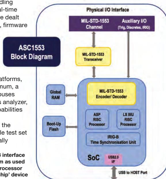
The ASC1553 interface block diagram as used by the dual processor 'system-on-chip' device in the connector
