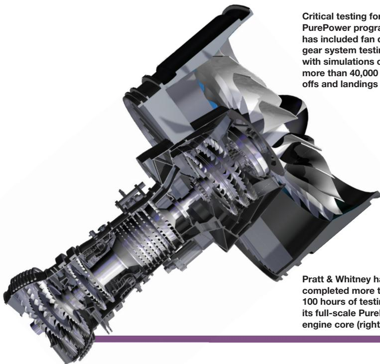
Critical testing for the PurePower program, has included fan drive gear system testing with simulations of more than 40,000 take-offs and landings
