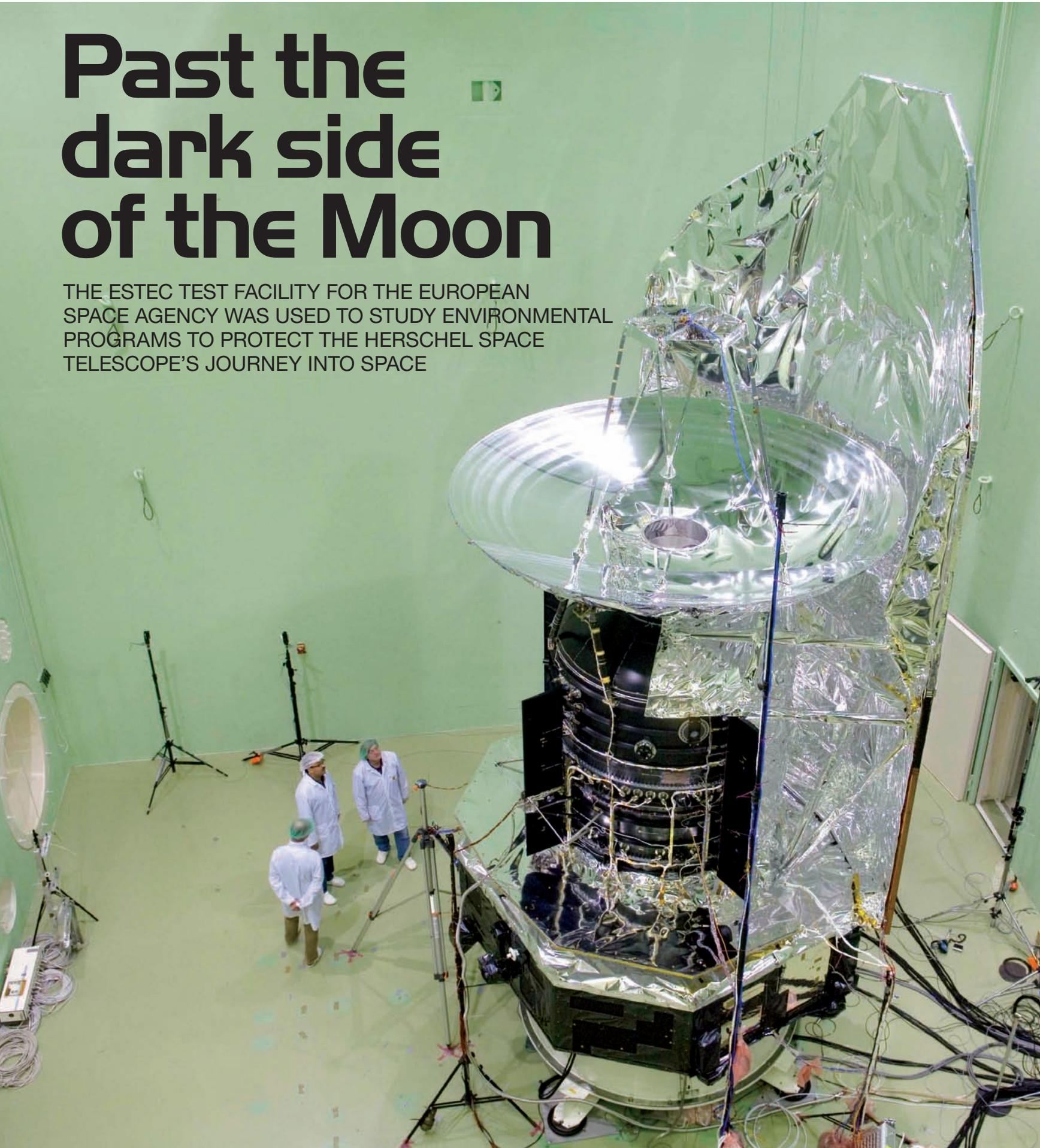
A typical test, the Herschel is prepared for lateral sine vibration along its X-axis in the frequency range 4-100Hz. For this vibration test, the flight-model spacecraft was fastened on electrodynamic shakers in the ESTEC test center. Starting at 4Hz, the shaker frequency steadily increased to 100Hz over a period of about 80 seconds
