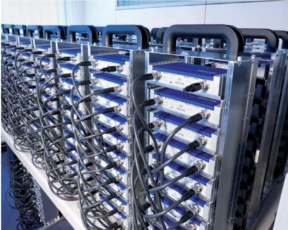
**Left: Installation comprising 400 CANHEAD modules for a 4,000-channel system**
