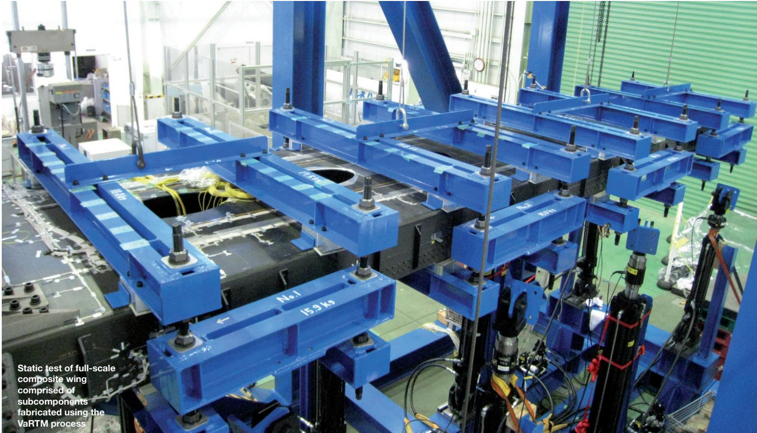
Static test of full-scale composite wing comprised of subcomponents fabricated using the VaRTM process
