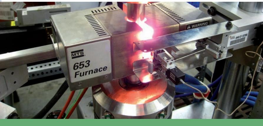
**In situ mechanical testing of thermal barrier coatings (above). Elevated temperature low-cycle fatigue (LCF) testing (left). Photos courtesy: University of Central Florida**
