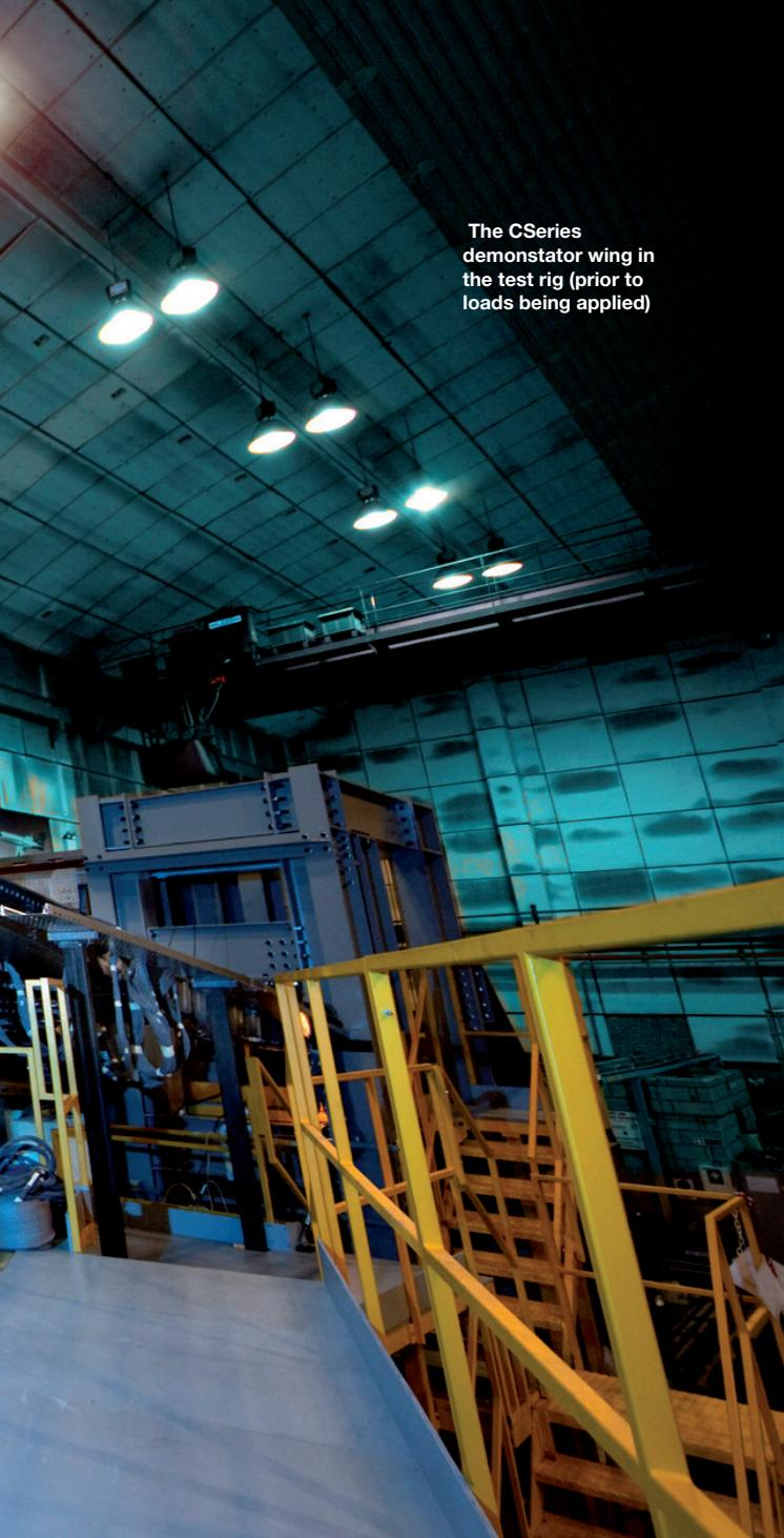
The CSeries demonstrator wing in the test rig (prior to loads being applied)
