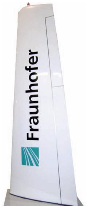
Far right: Mock-up of a 4m tall composite wing with over 40 embedded and surface applied sensors
