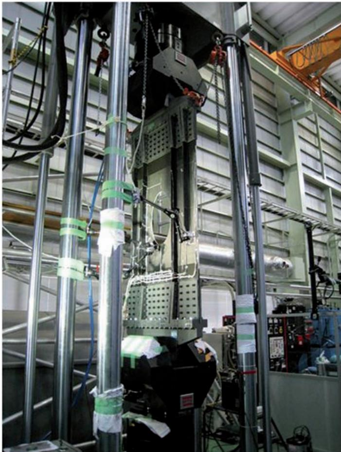
**Left: Fatigue test of composite subcomponent fabricated using the VaRTM process**
