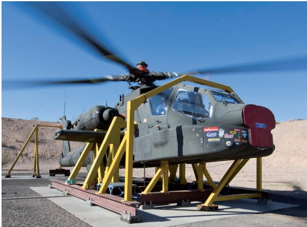
**The Block III Ground Test Vehicle running in test pit in specially designed test rig**
