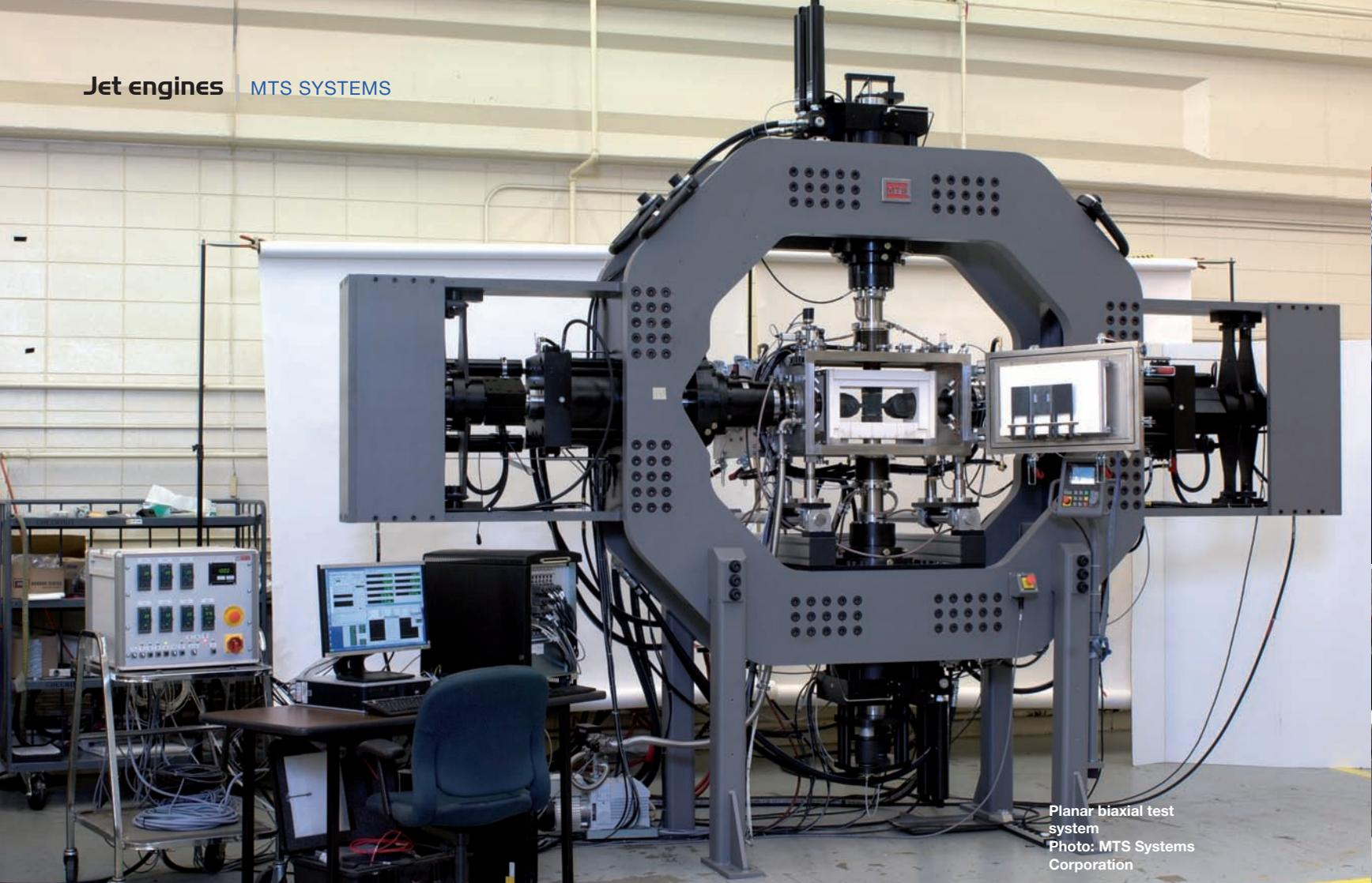
Planar biaxial test system
