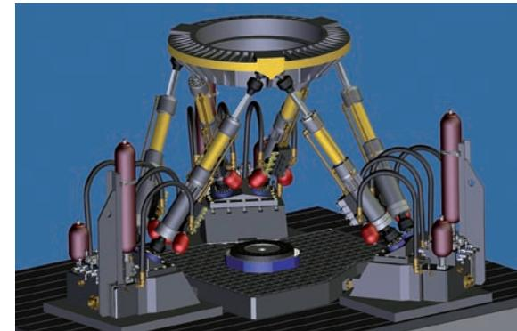
Hexapod testbed, nose-gear testbed and automated test system for rims
