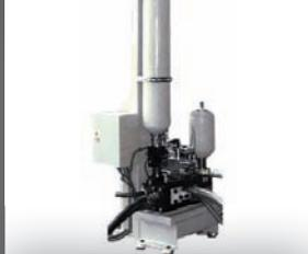
Hydraulic power supply with separate filter and cooling circuit resulting in a great durability of the servo valves
