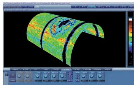
Left: Computer 3D image showing cylinder impact
