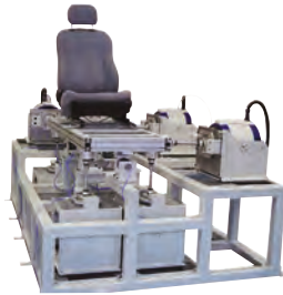
6 degree of freedom vibration test system
