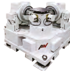
Multi-axis vibration test system
