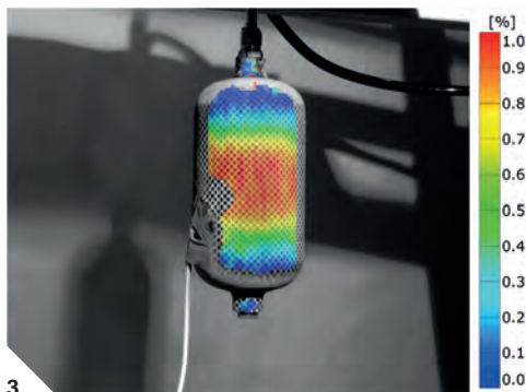
3 // Hoop strains superimposed over the composite overwrapped pressure vessel (COPV) during a burst test. These strains are measured using full-field strain mapping
