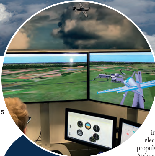
5// Siemens' real-time simulation environment for an electric propulsion system, based on a Siemens LMS solution interfaced to a test bench
