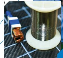
1,2 // Carbon fiber with embedded circuitry to detect cracks, developed at the Center for Composite Materials in Moscow
