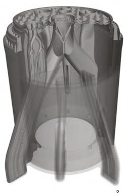
The new CT algorithms ensure optimum image resolution with a larger field of view. The innovative ScanExtend feature enables horizontal field-of-view extension and is suitable for scanning larger objects or for maximum magnification of smaller parts. The scan is performed in one rotation of the test part and reconstructed without artifacts. This saves time compared with current algorithms.
