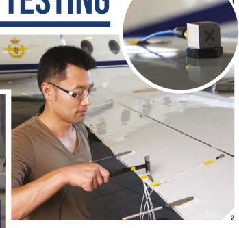
1 // Triaxial ICP modal accelerometer wing mounted with an electrically isolated base
