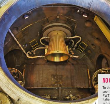
is enough to light up a town of 80,000 people," he says. "It can generate the world's largest hypersonic plasma jet as a result of its maximum nozzle exit diameter of 2m (6.5ft), which enables the testing of real-scale models with a front diameter of 60cm (23in) and over. The footprint of the facility, including its subsystems and auxiliaries, is incredibly large. The size can only really be conveyed by satellite imagery."
