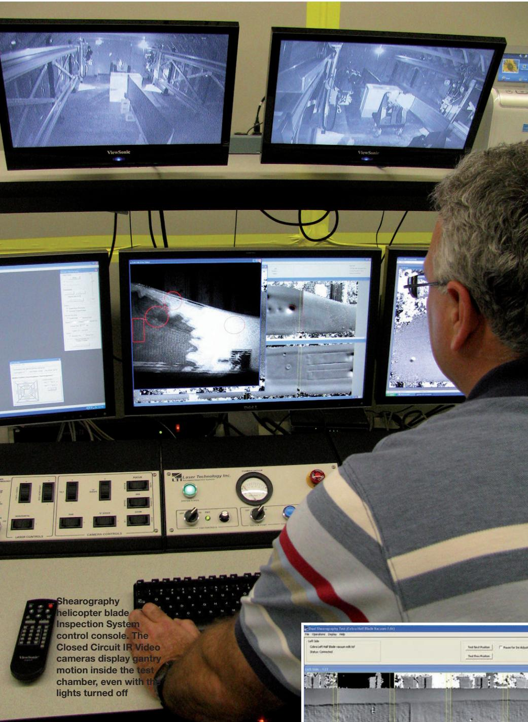
Shearography provides inspection results in minutes, without any part contamination or wetting of the test part. System features such as teach/learn part-scan programming; automatic image stitching, creating a single image of the entire part; image analysis and defect measurement tools; and automated operation are comparable to c-scan systems. In addition, shearography cameras do not require part contour following because the part imaging is effective even as steep angles.
