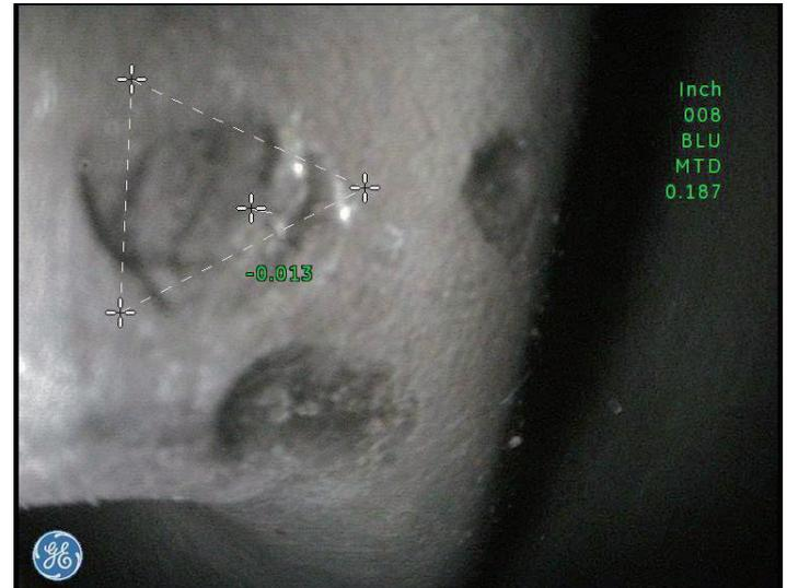
Cursor positioning with phase measurement
