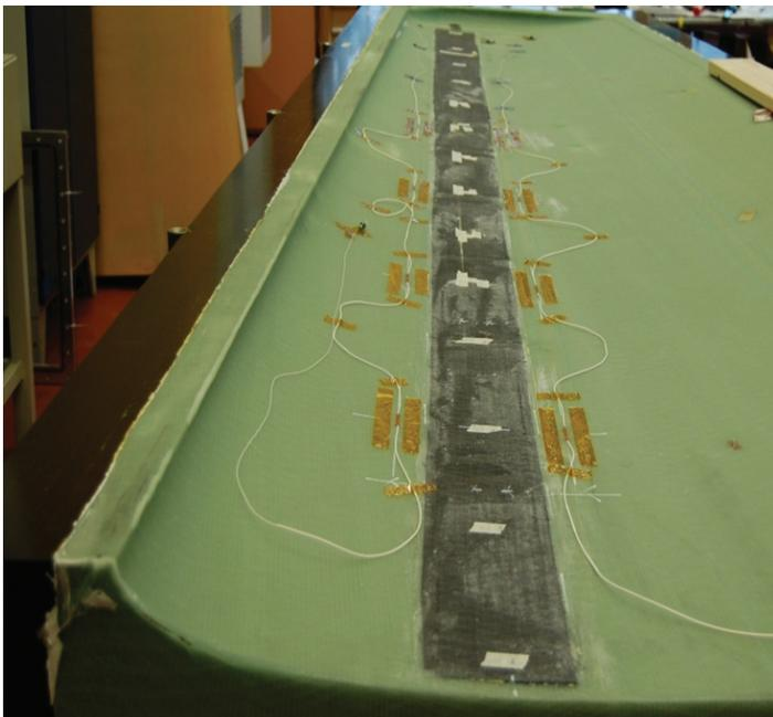
**'Intelligent' sensor-equipped composite structures require a sophisticated combination of sensor and manufacturing technology, as well as data acquisition and analysis software**
