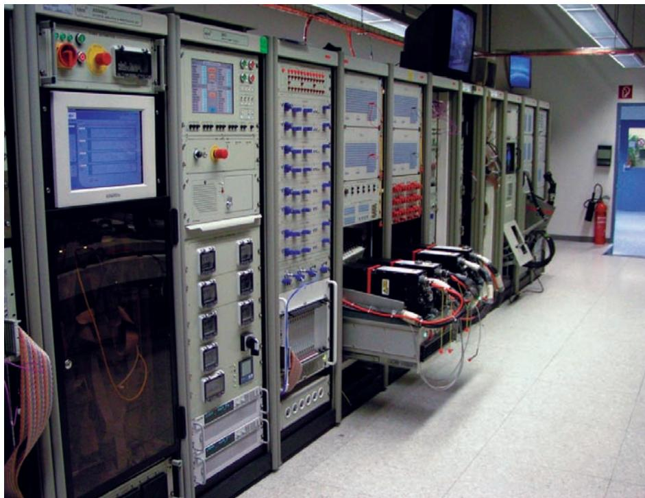
**Above: Large test system, comprised of several racks of equipment, for integration testing of aircraft electronics**
