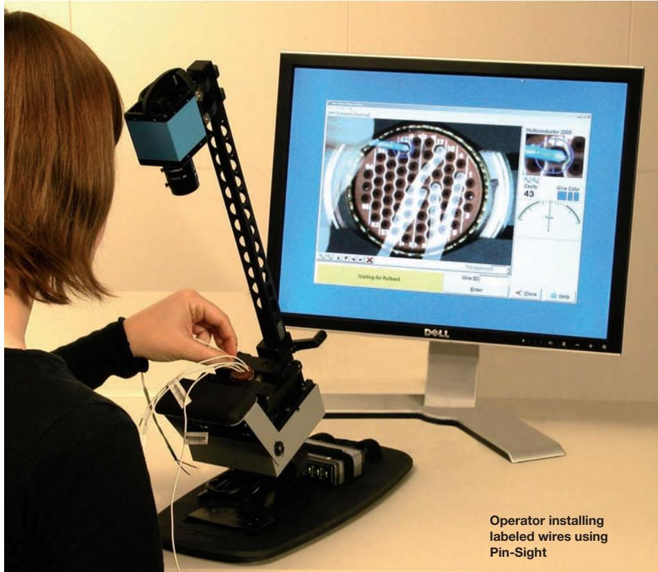
Operator installing labeled wires using Pin-Sight
