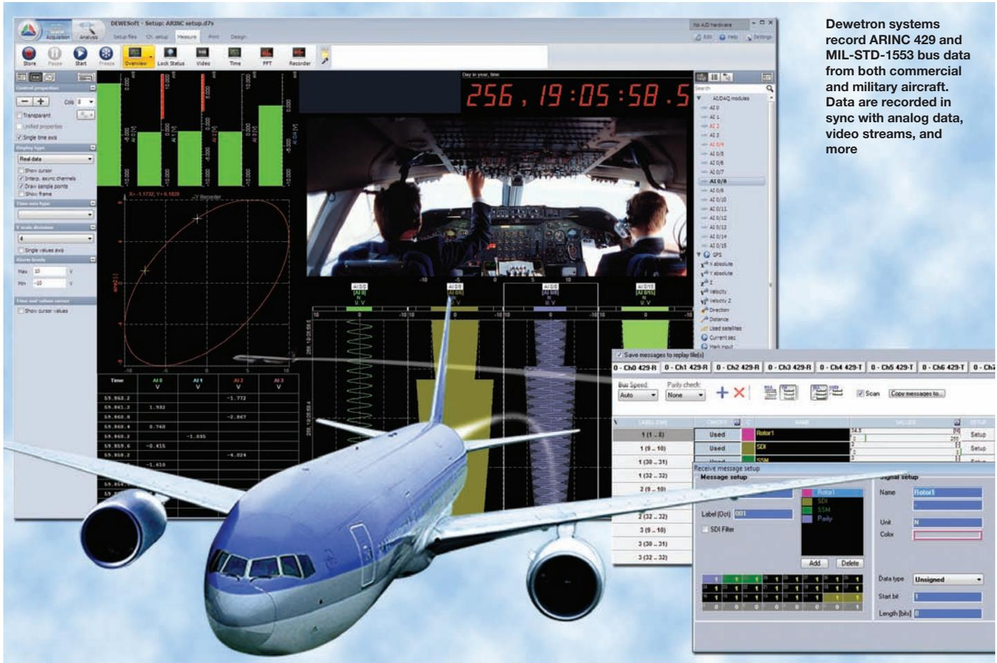
Dewetron systems record ARINC 429 and MIL-STD-1553 bus data from both commercial and military aircraft. Data are recorded in sync with analog data, video streams, and more
