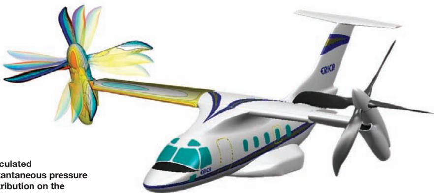
Calculated instantaneous pressure distribution on the ERICA rotor and wing
