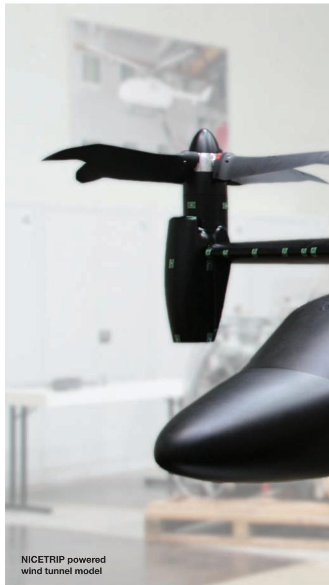
NICETRIP powered wind tunnel model
