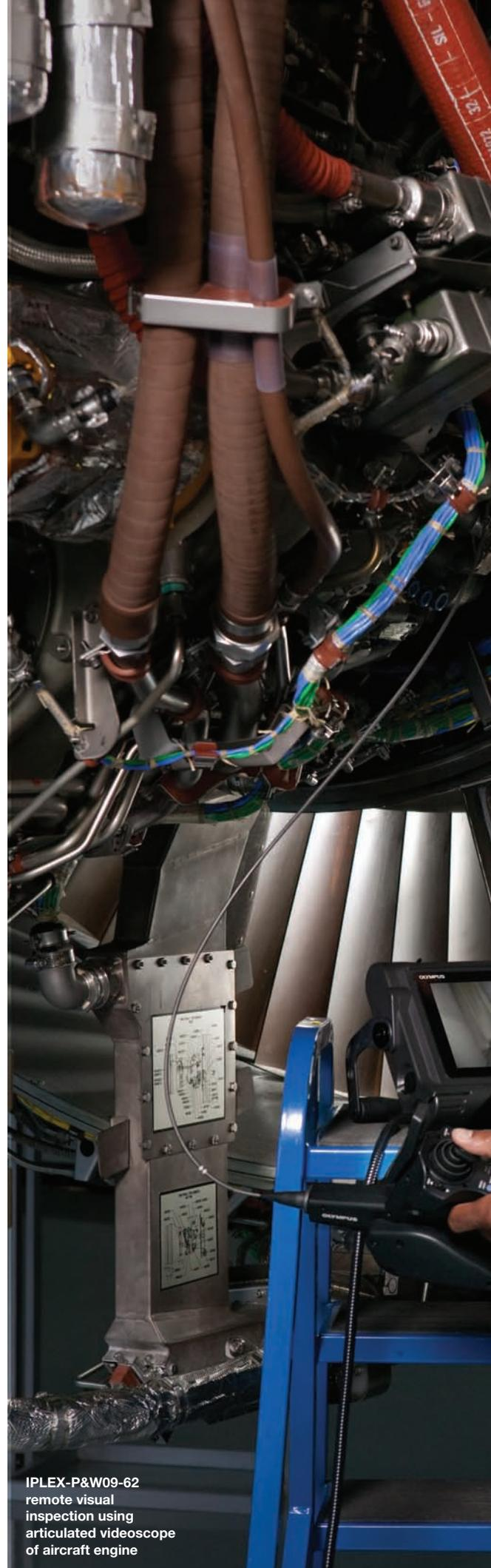
IPLEX-P&W09-62 remote visual inspection using articulated videoscope of aircraft engine
