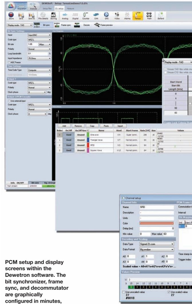
PCM setup and display screens within the Dewetron software. The bit synchronizer, frame sync, and decommutator are graphically configured in minutes, and data are easily displayed in a wide variety of formats during acquisition to disk
