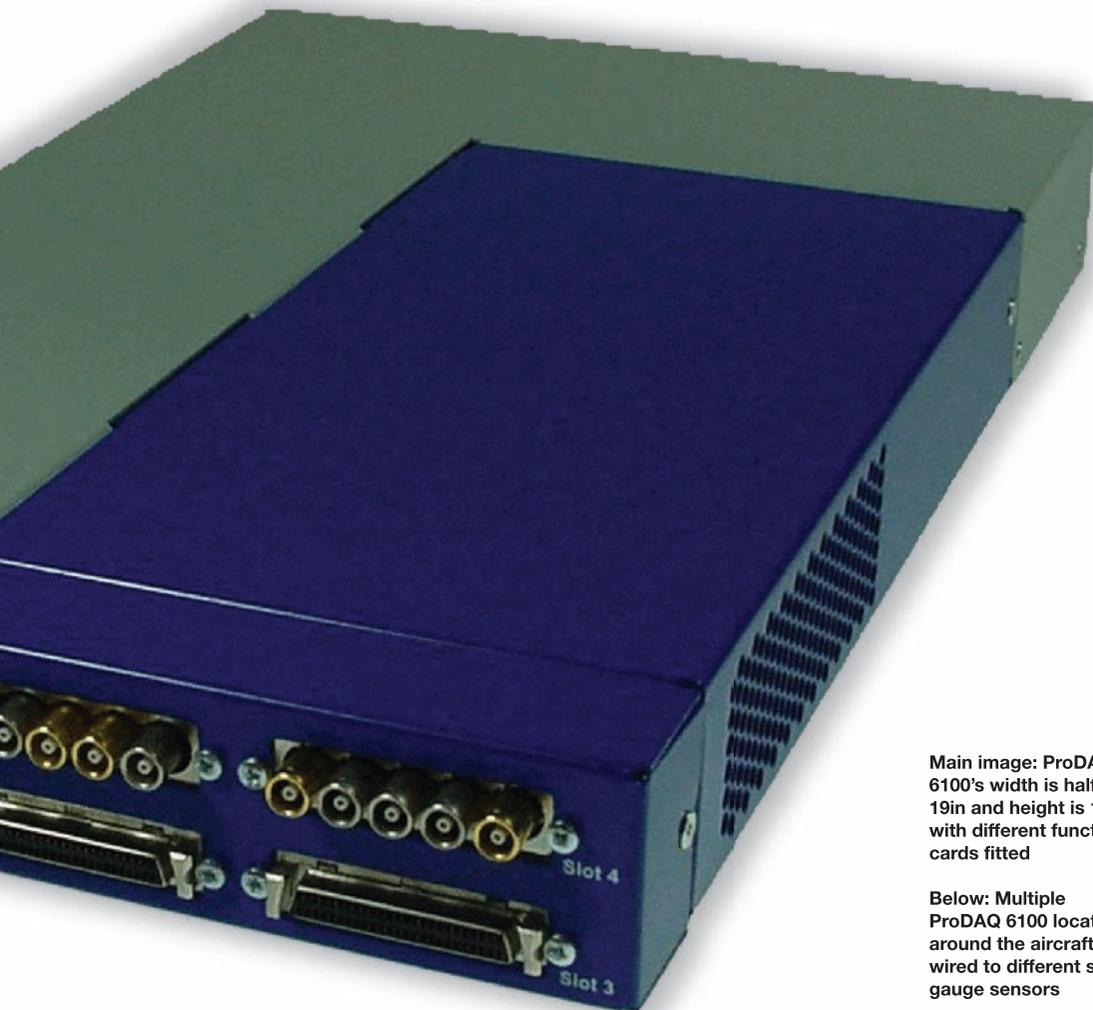
**Main image: ProDAQ 6100's width is half of 19in and height is 1U with different function cards fitted**
