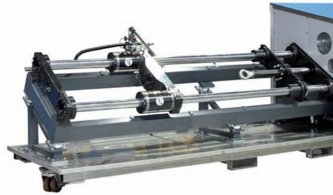
Modular hydraulic test stand for non-rotating components
