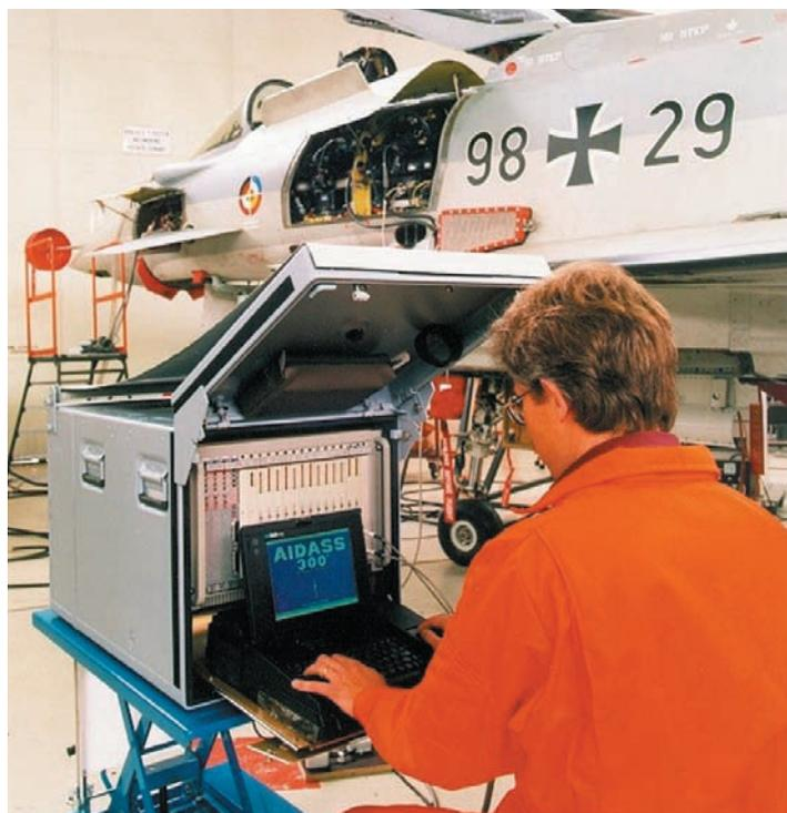
**Left: Ruggedized portable aircraft ground equipment for on-aircraft diagnostics**
