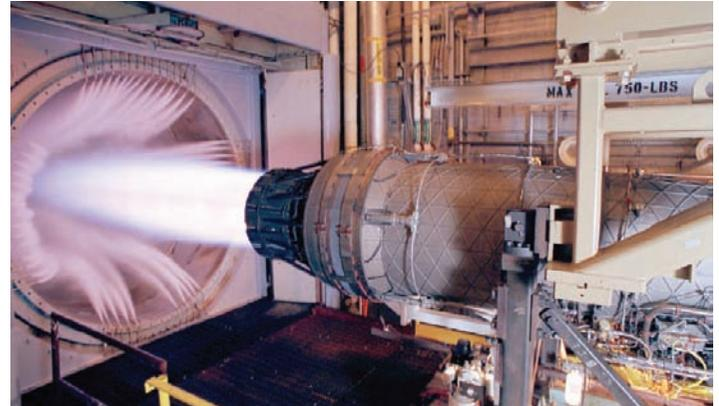
**Above: The F100 Engine for the F-15 and F-16 being tested in SL-2**
