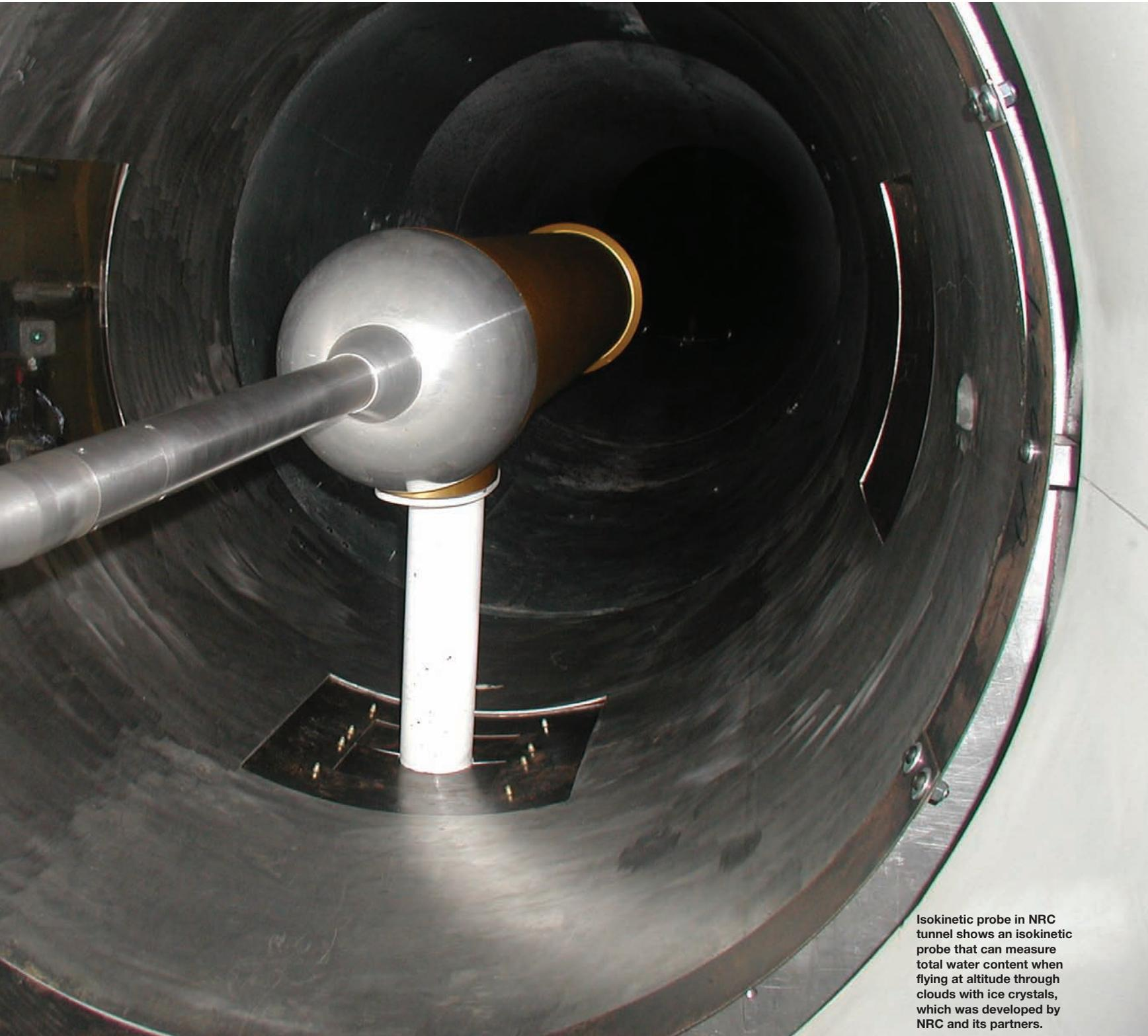
Isokinetic probe in NRC tunnel shows an isokinetic probe that can measure total water content when flying at altitude through clouds with ice crystals, which was developed by NRC and its partners.
