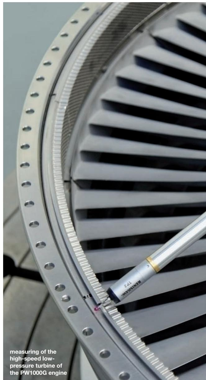
measuring of the high-speed low-pressure turbine of the PW1000G engine
