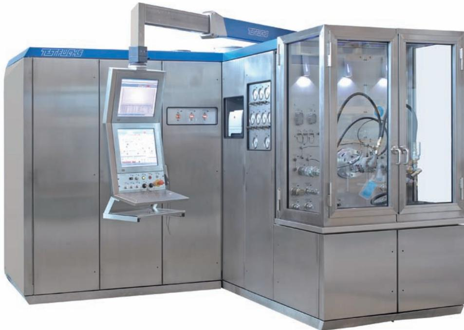
Undertaken in consultation with the customer, the development of the LMP300 will be the most comprehensive version of the company's aircraft-power generation components-testing equipment. This test bench is capable of testing all power-generation components (IDG, generators, CSD) installed on various aircraft types from the Embraer and Q400 up to the A380 and B787.
