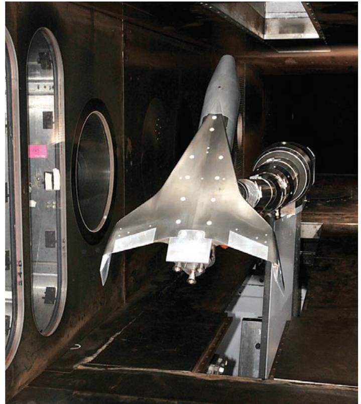
Fully-reusable access to space technology proof-of-concept launch vehicle in Tunnel A
