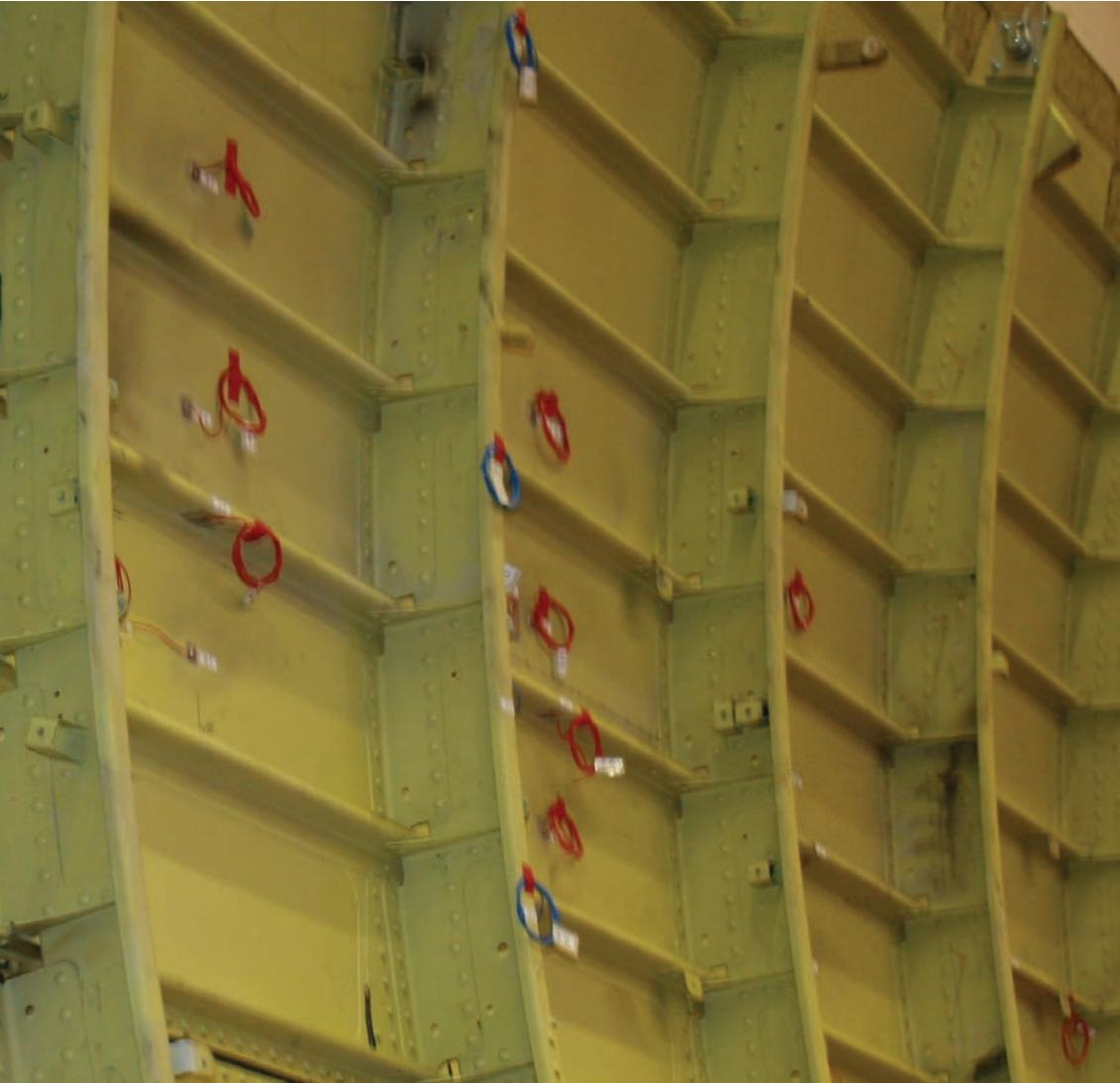
**Left: Structural health monitoring for a fuselage panel. (Fraunhofer LBF)**
