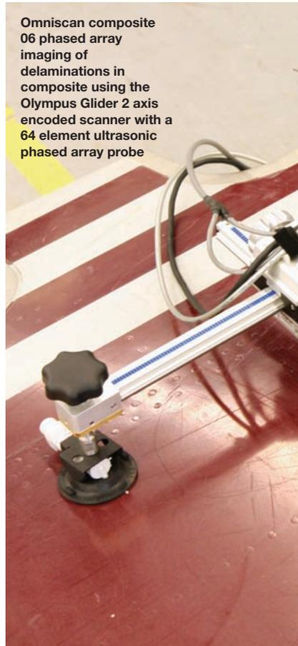
Omniscan composite 06 phased array imaging of delaminations in composite using the Olympus Glider 2 axis encoded scanner with a 64 element ultrasonic phased array probe
