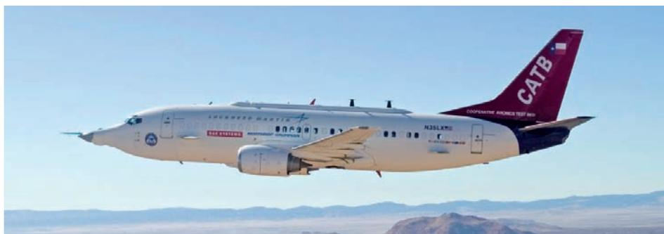
A 27ft spine, running on top of the fuselage, contains two more of the six total DAS sensors; the global positioning system receiver; antennas associated with UHF, VHF, and satellite communications; and several datalinks, including assemblies and interface units associated with the F-35's multifunction advanced datalink (MADL). This sophisticated datalink enables the aircraft to communicate within and between flights and share a common view of the battle space.
