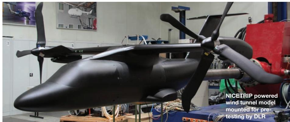
NICETRIP powered wind tunnel model mounted for pre-testing by DLR
