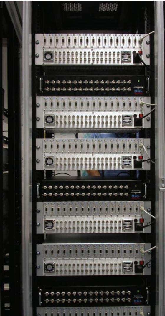
Left: Synchronised dynamic data acquisition on hundreds of channels, using modular components and standard network infrastructure
