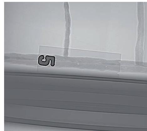
**“Even small differences in contrast caused by small casting flaws become clearly visible”**
