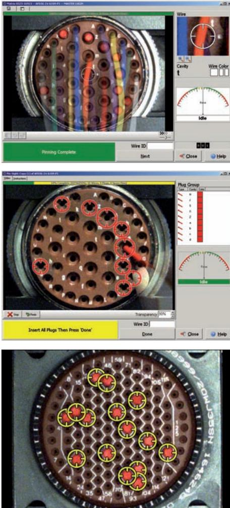
Above: guided insertion of sealing plugs. Quick and easy inspection that all seal plugs are inserted correctly. Transparency setting lets you "see through" installed wires
