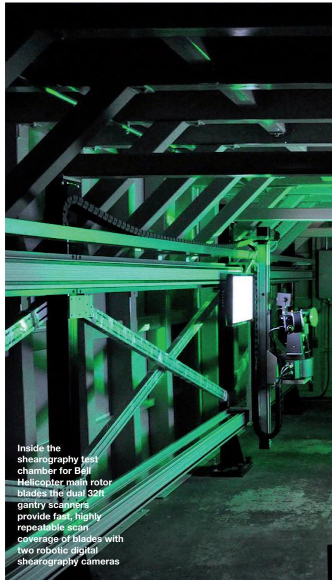
Inside the shearography test chamber for Bell Helicopter main rotor blades the dual 32ft gantry scanners provide fast, highly repeatable scan coverage of blades with two robotic digital shearography cameras
