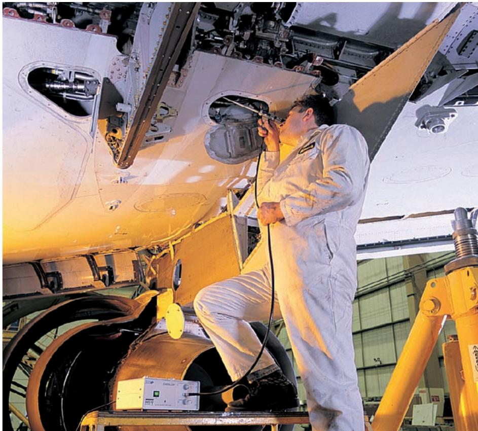
borescope's data capture system. Finally, a hardcopy report is produced with a convenient click-to-report feature.
