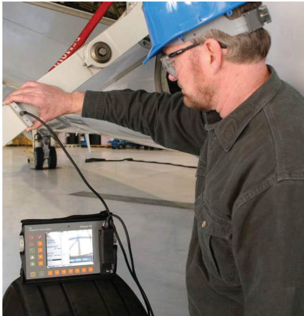
TOP: The Bondtracer device for detecting and sentencing minor composites damage
