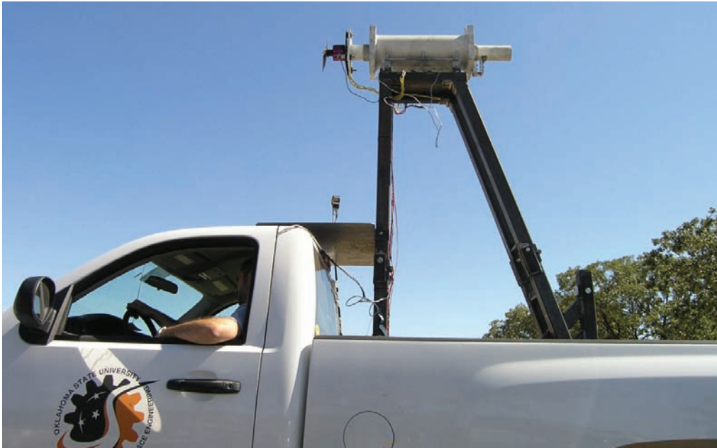
ABOVE: Propulsion testing in relevant environments is critical – to this end, propellers and motors can be tested on an automotive mounted dynamometer prior to flight tests
