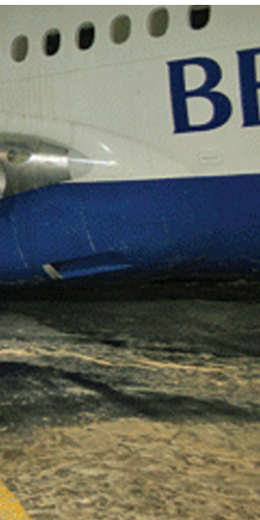
ABOVE: Speedbird 38 landed short of the Heathrow runway in 2008. The cause was found to be ice crystals in the fuel clogging the fuel/oil heat exchanger
