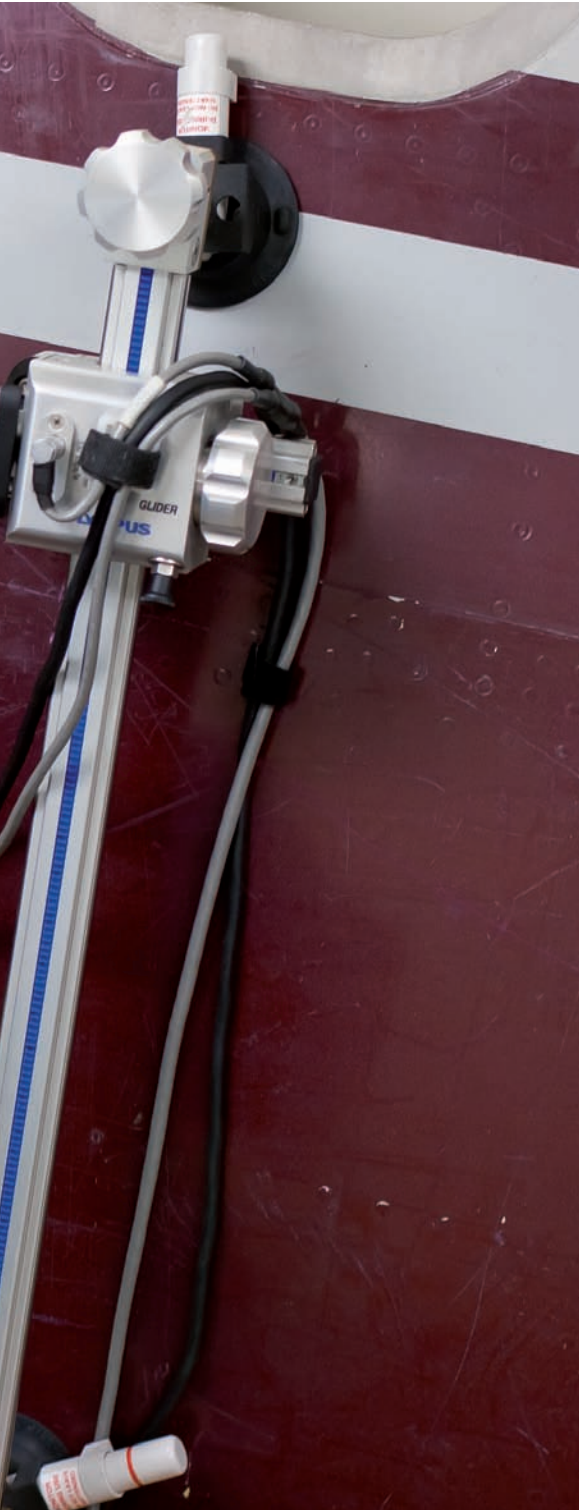
ABOVE: Element steps of a linear array, Linear array probe with wedge
