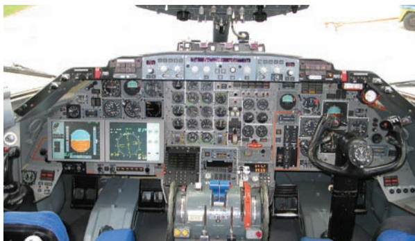
BELOW: The cockpit of ATTAS: The left-hand side of the cockpit where the experimental pilot sits is equipped with configurable displays and a side-stick. The safety pilot sits on the right seat and sees the unmodified original cockpit of the VFW 614
